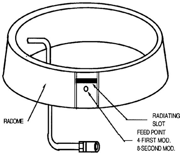
Figure 3- Modified Antenna
