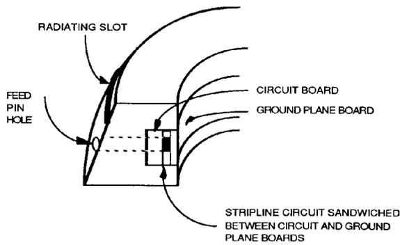
Figure 2- Integrated Stripline Feed Network
