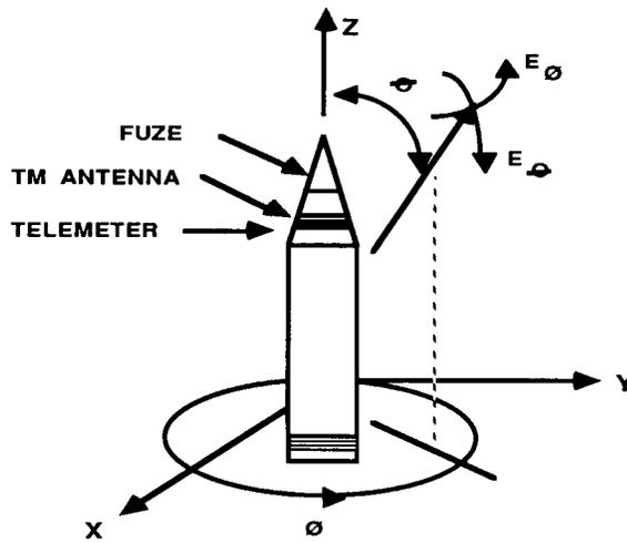
Figure 1 - Coordinate System for Pattern Measurements
