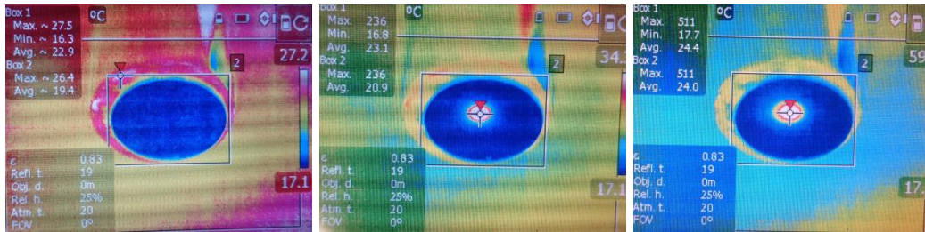
Figure 5.6 Pump spot temperature experience in thin disk.
