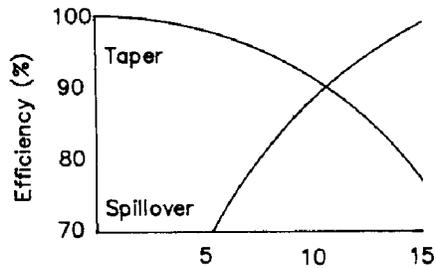
Figure 1. Edge Illumination (dB) Taper and Spillover Losses
