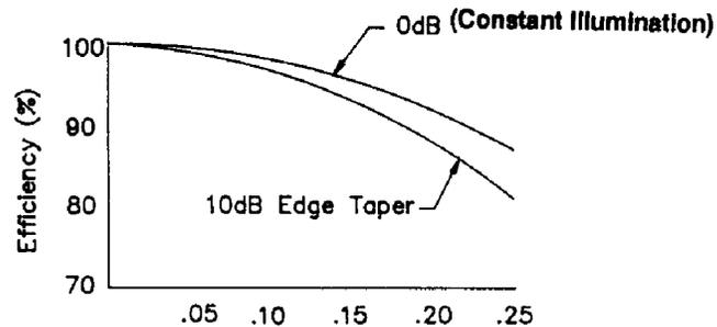
Figure 2. Losses Due to Central Blockage Ratio (Df/D)\*
