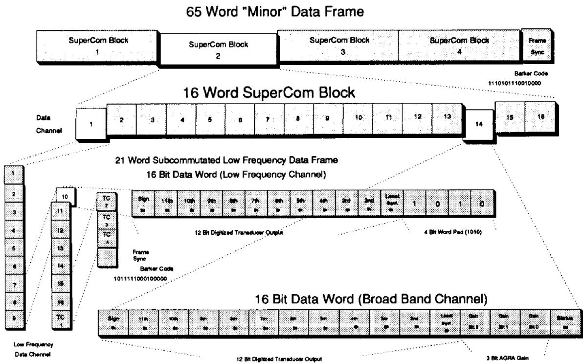
Figure 4. PCM Frame Structure
