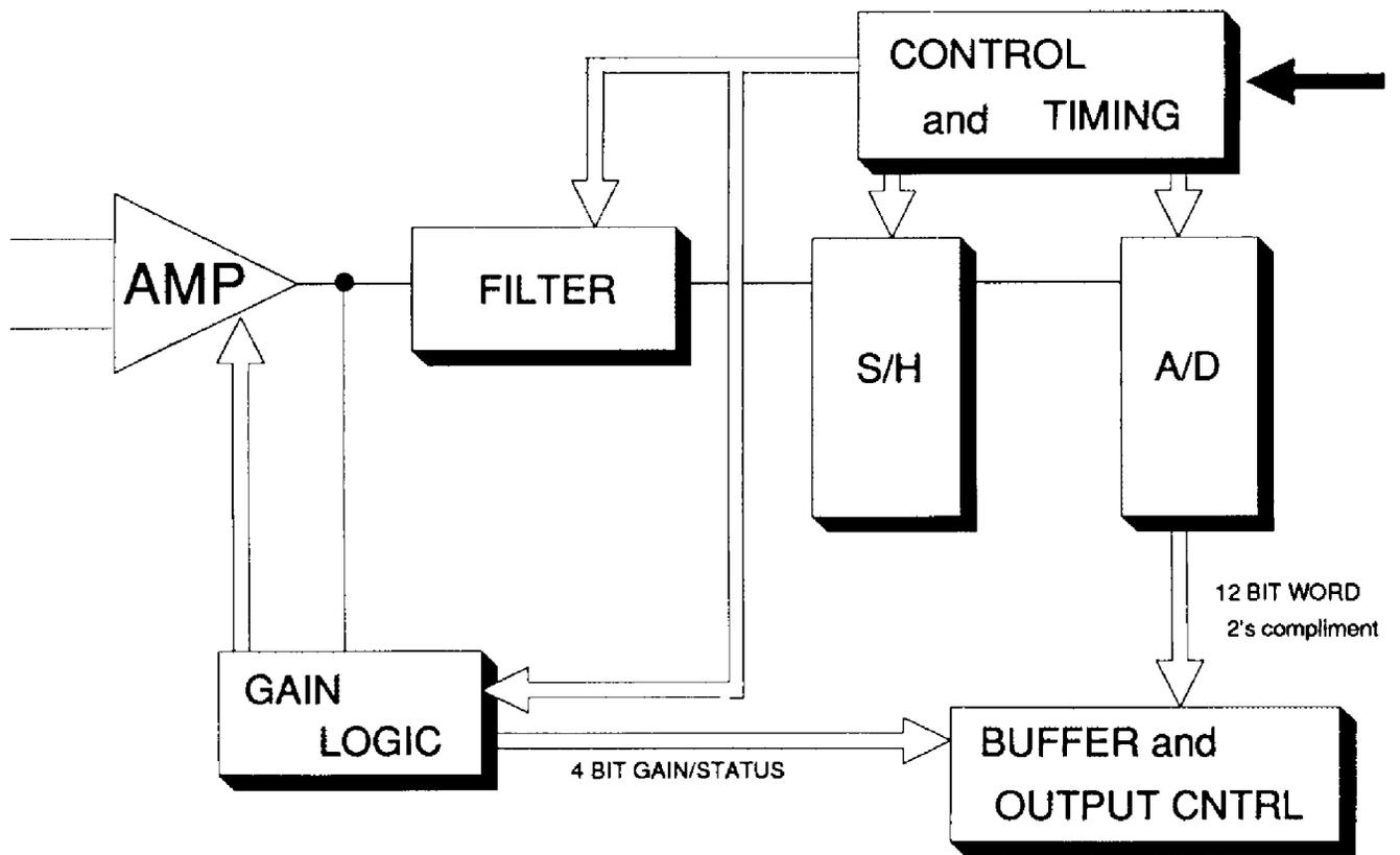
Figure 3. Automatic Gain Ranging Amplifier (AGRA)
