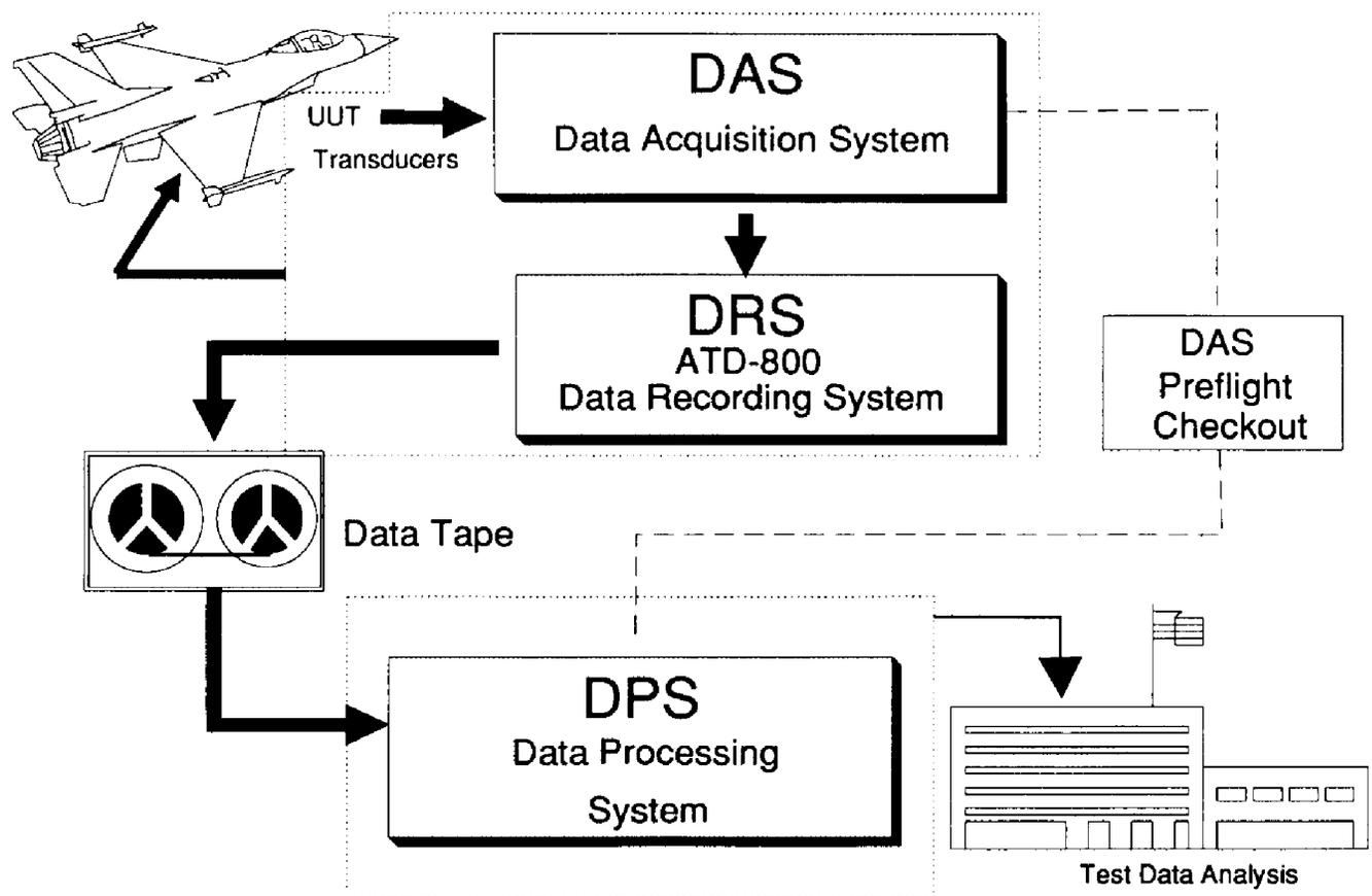
Figure 1. Digital Data Acquisition and Processing System
