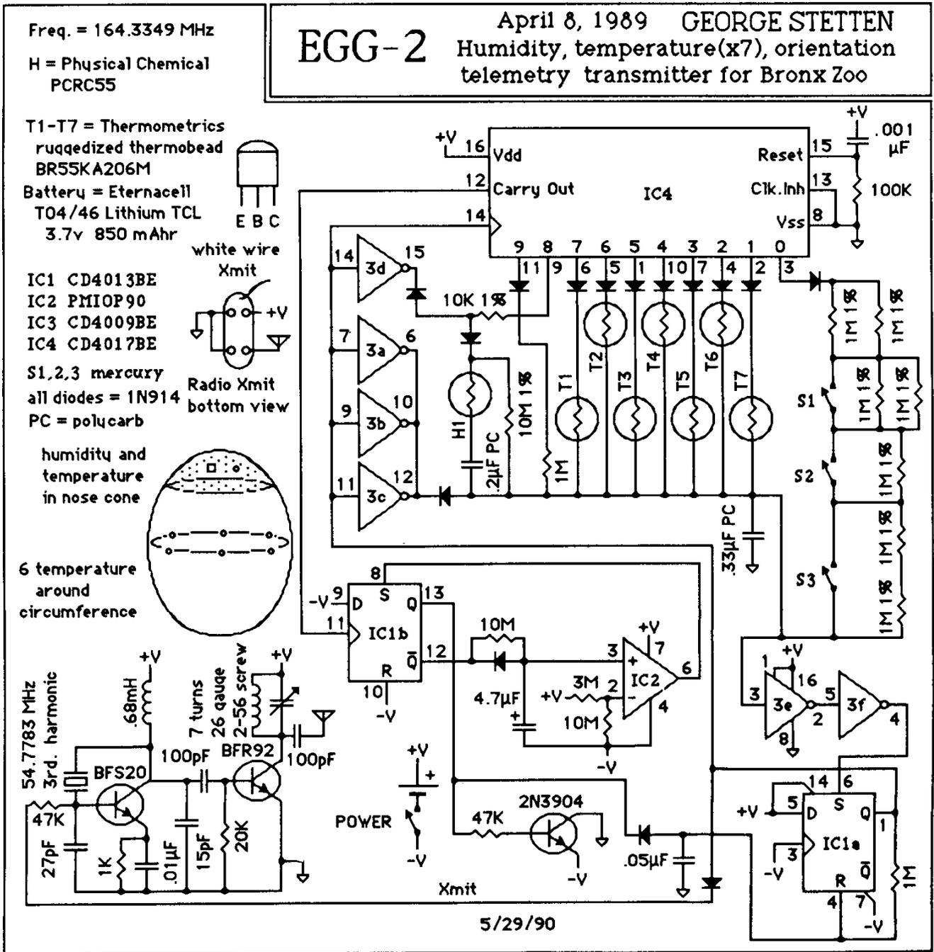
**Figure 2 : Schematic of EGG-2 Telemetry Transmitter**
