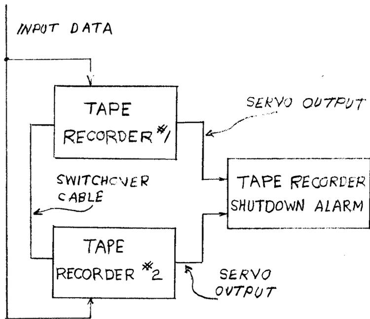
**FIGURE #3 - ALARM CONNECTED TO TWO RECORDERS**
