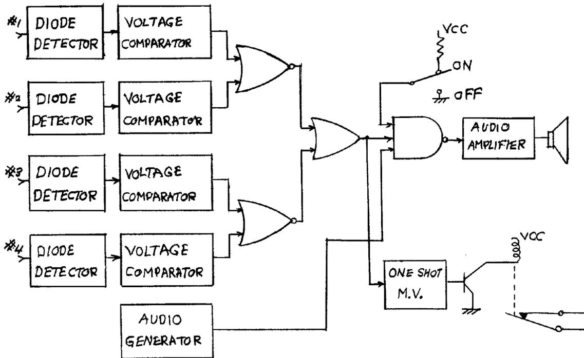
**FIGURE #7 - ALARM FOR USE WITH FOUR RECORDERS**
