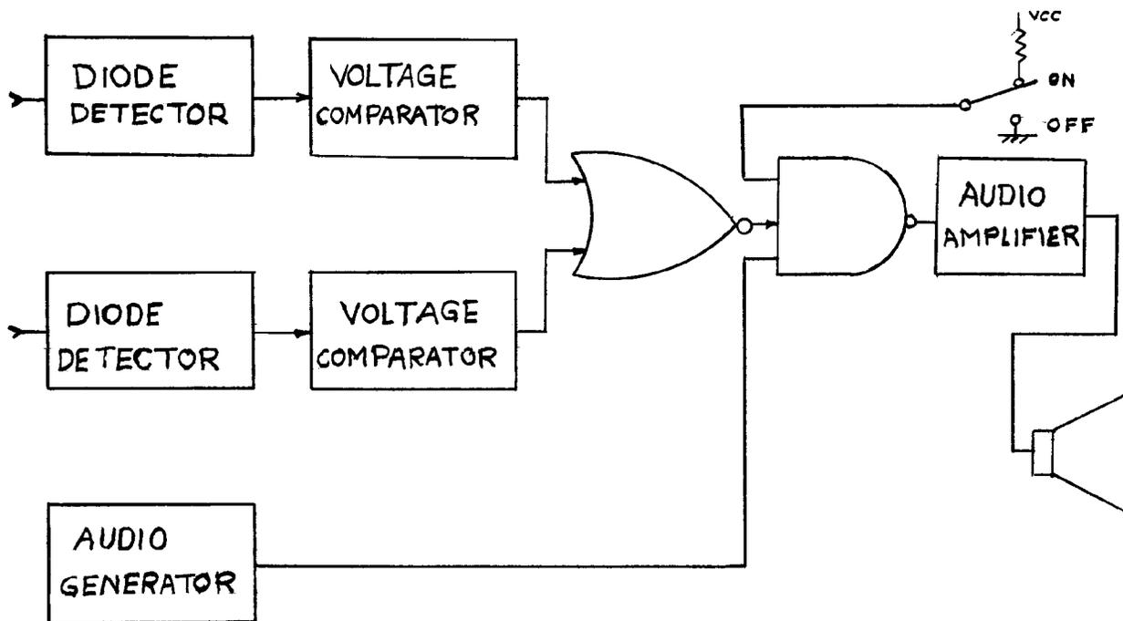
**FIGURE #2 - TAPE RECORDER SHUTDOWN ALARM**
