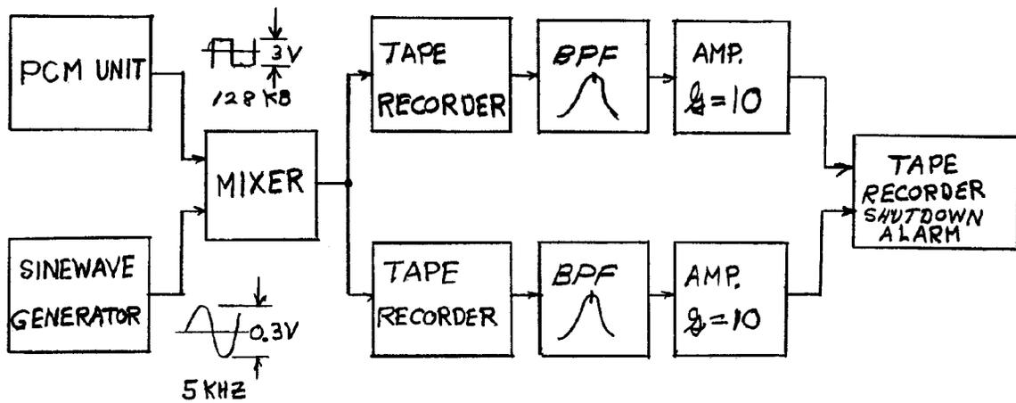
**FIGURE #9 - ALARM USED WITH TAPE RECORDERS THAT DO NOT RECORD SERVO SIGNALS**
