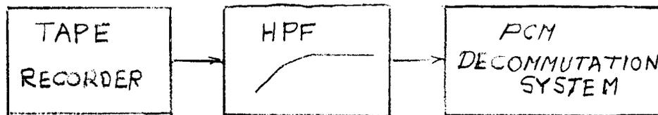
**FIGURE #10 PLAYBACK OF PCM DATA MIXED WITH ALARM SIGNAL**
