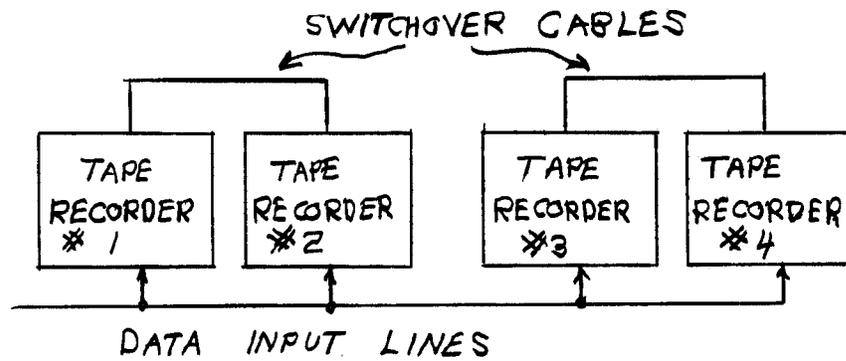
**FIGURE #6 - USE OF REDUNDANT RECORDING TO PREVENT DATA LOSS**
