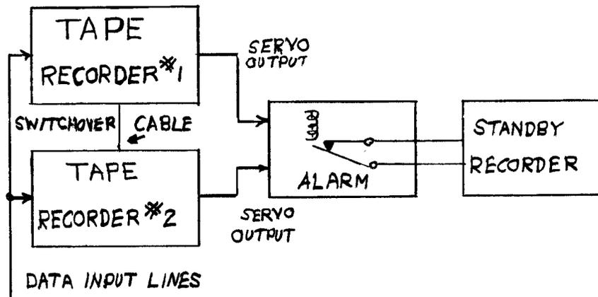
**FIGURE #5 - ALARM CONNECTED TO STANDBY RECORDER**
