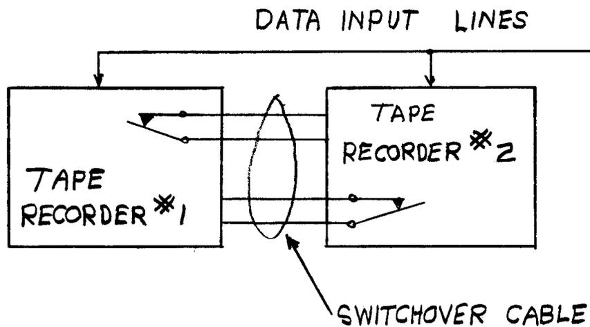
**FIGURE #1 - TAPE RECORDERS CABLED TO SWITCHOVER AT END OF RUN**
