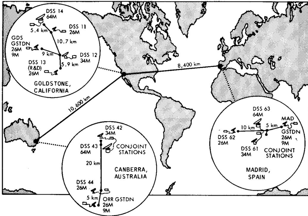
**FIGURE 3. NASA DEEP SPACE NETWORK COMPLEXES WITH COLOCATED GSTDN STATIONS**
