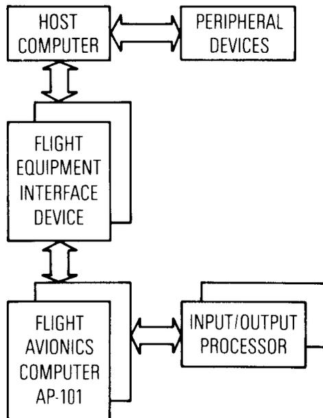
**Figure 11. Data Load Preparation System**
