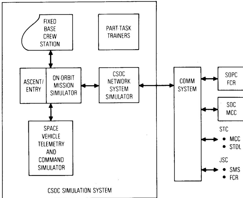
**Figure 12. CSOC Simulation System Overview**
