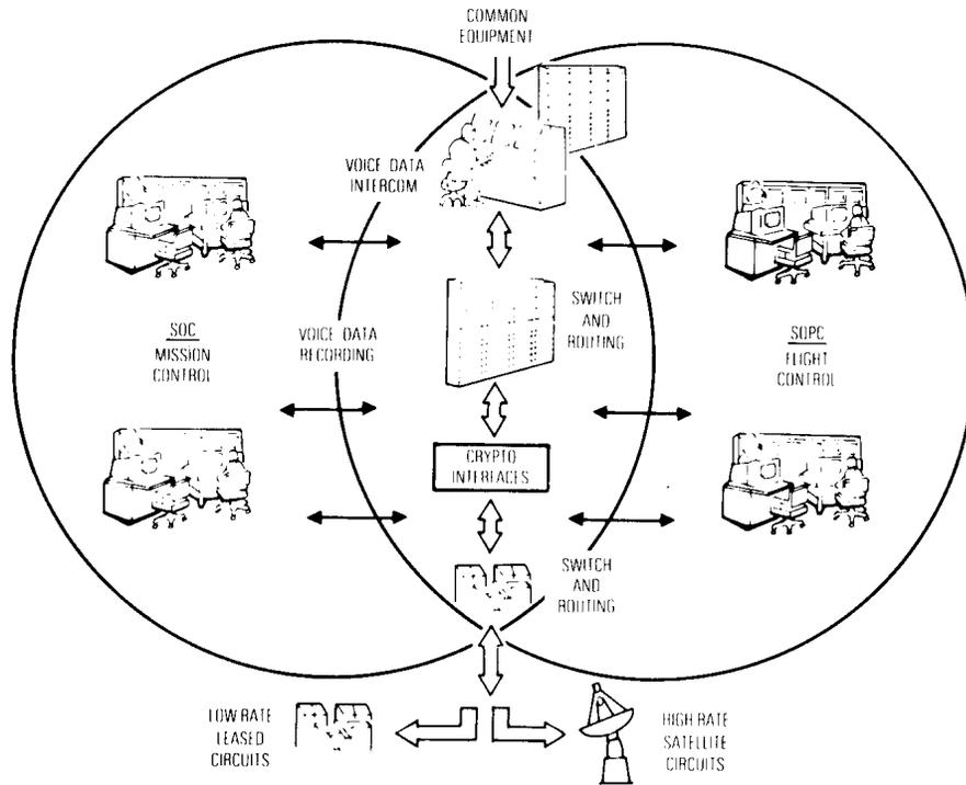
**Figure 14. CSOC Internal Communications**
