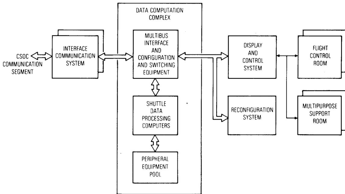
**Figure 13. Flight Control Element**
