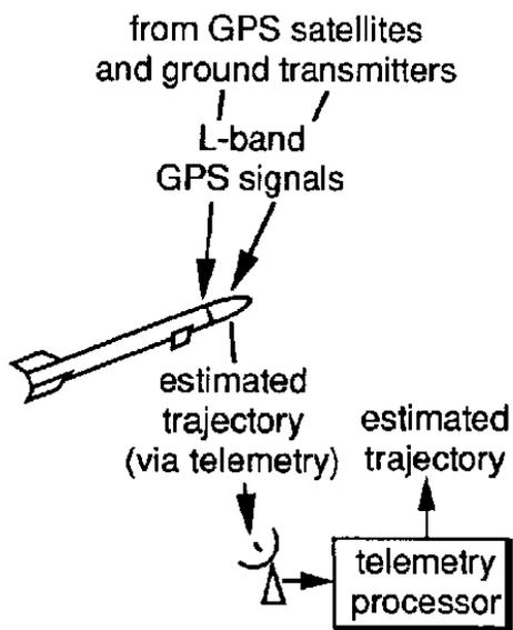
**Figure 1. On-board GPS Receiver.**
