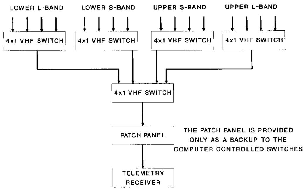
ALL SIGNALS HAVE BEEN DOWN CONVERTED TO 215-320 MHz
