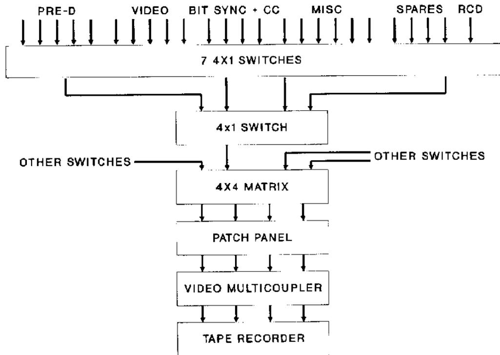
**Figure 3.** Recorder Input Switches (4 Tracks).
