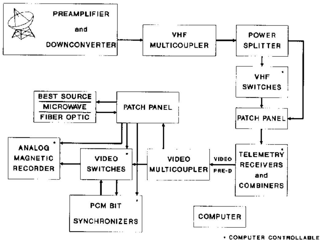
Figure 1. Receive and Record System Block Diagram.
