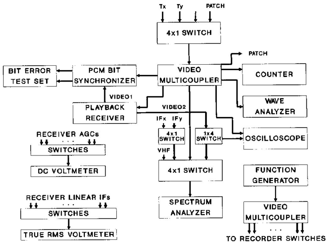
**Figure 5.** Station Test Equipment.
