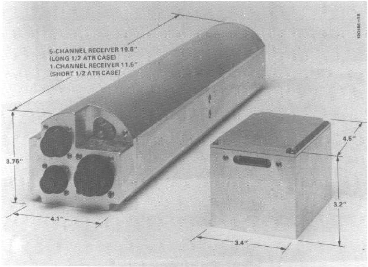
Figure 2. Advanced GPS Receiver
