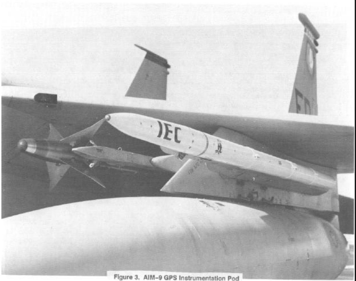
Figure 3. AIM-9 GPS Instrumentation Pod
