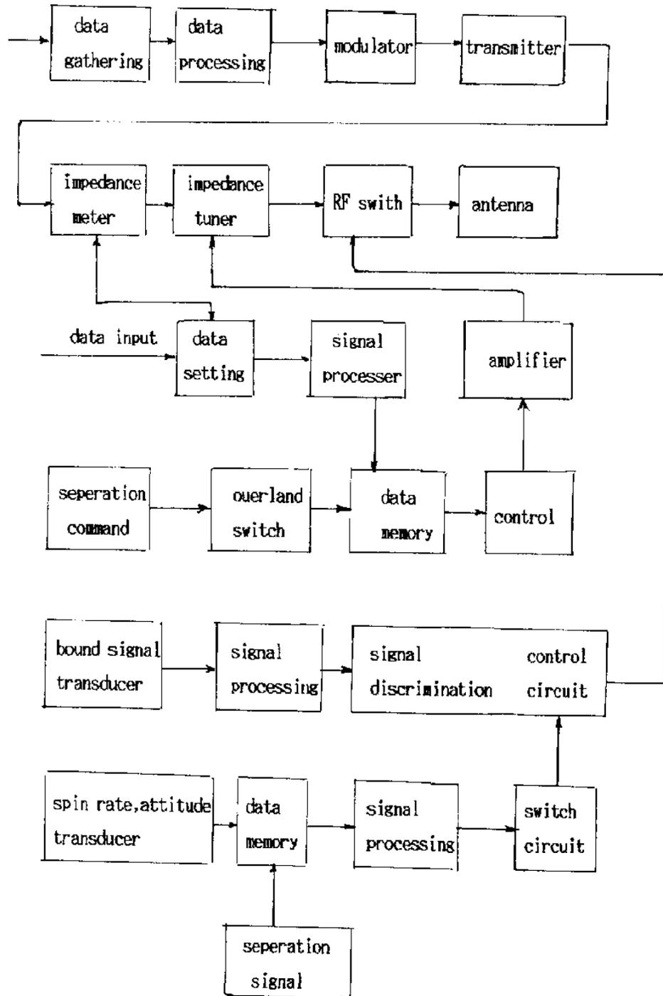
Picture 1. schematic block diagram of reentry telemetry system aboard
