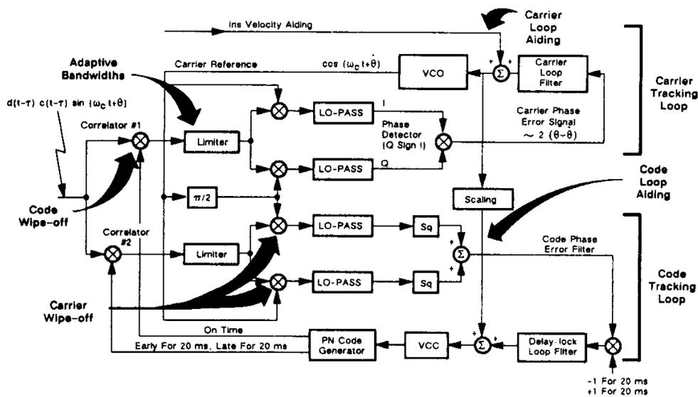
**Figure 1** GPS Receiver Functional Block Diagram - Coherent Mode
