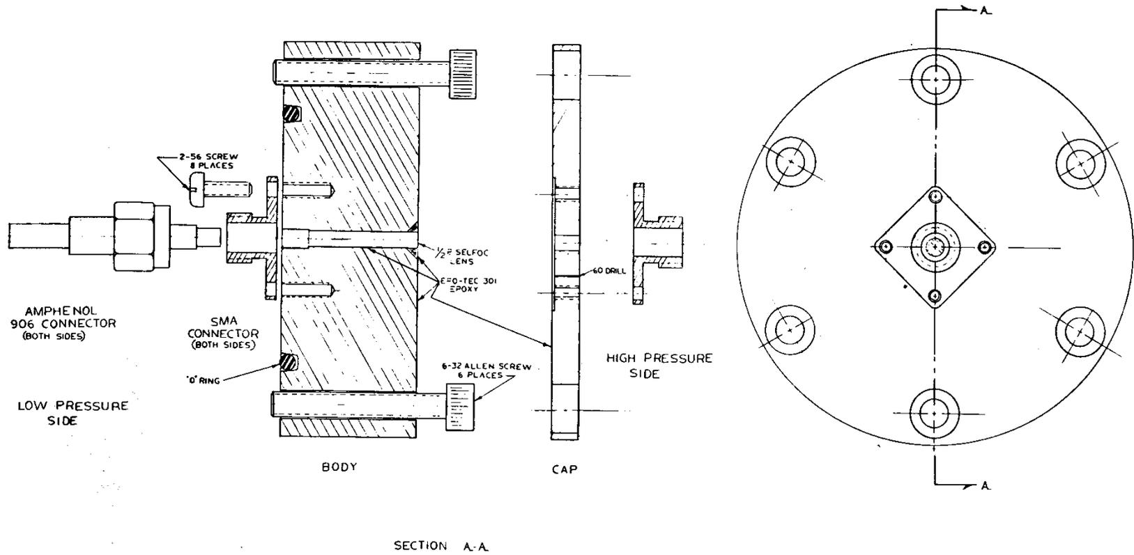
**Figure 11 - Fiber Optic penetrator assembly.**
