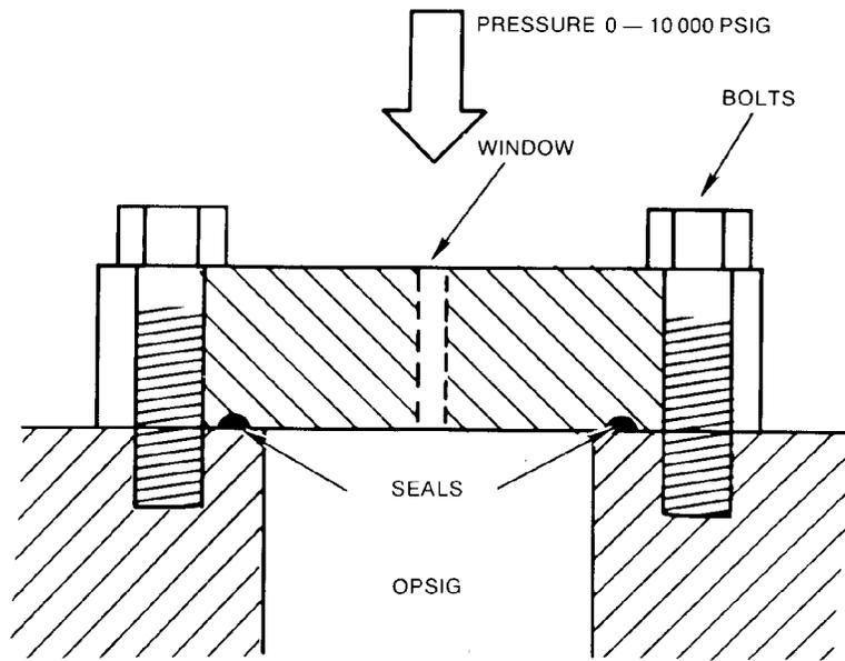
**Figure 9 - Plate covering a 1-inch diameter mounting hole, modeling considerations.**
