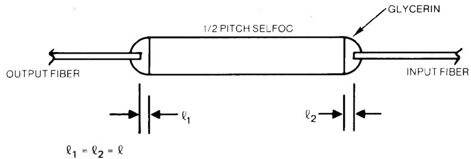
**Figure 6 - Experimental configuration employed to evaluate the insertion loss of SELFOC lens.**
