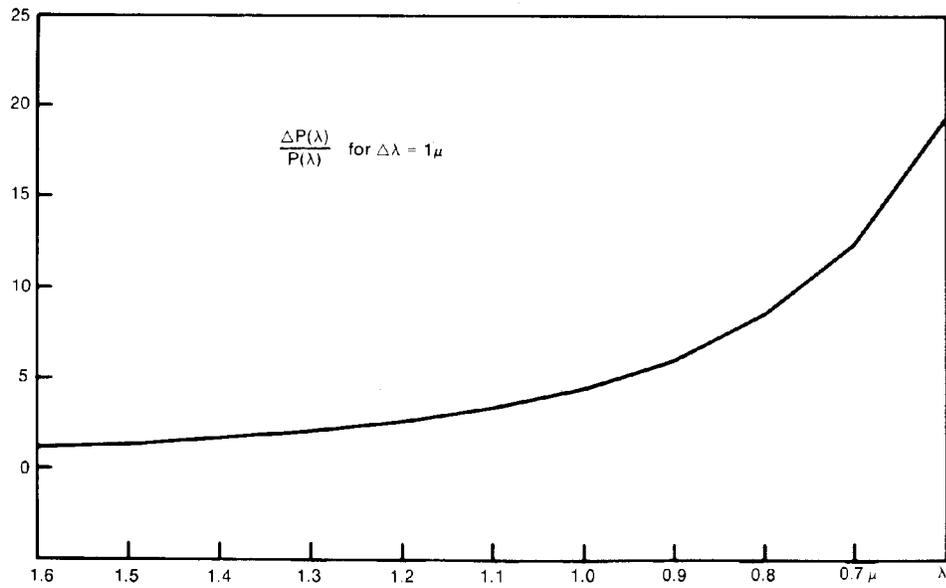
**Figure 5 - Chromatic pitch dependence vs wavelength for NSG type SLL/2mm SELFOC rod lens**
