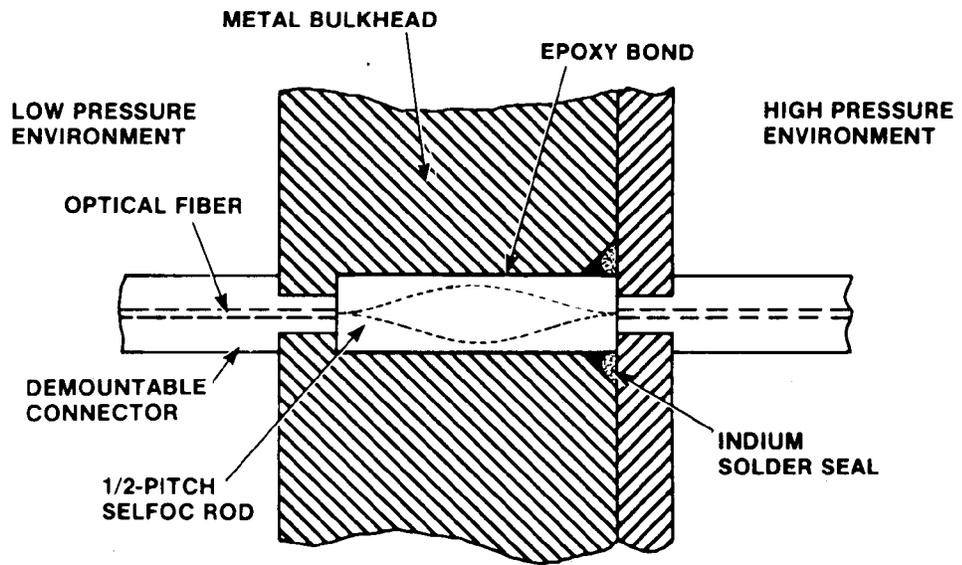
**Figure 1 - Schematic - Graded Refractive Index (GRIN) rod lens - combination pressure barrier and imaging device.**
