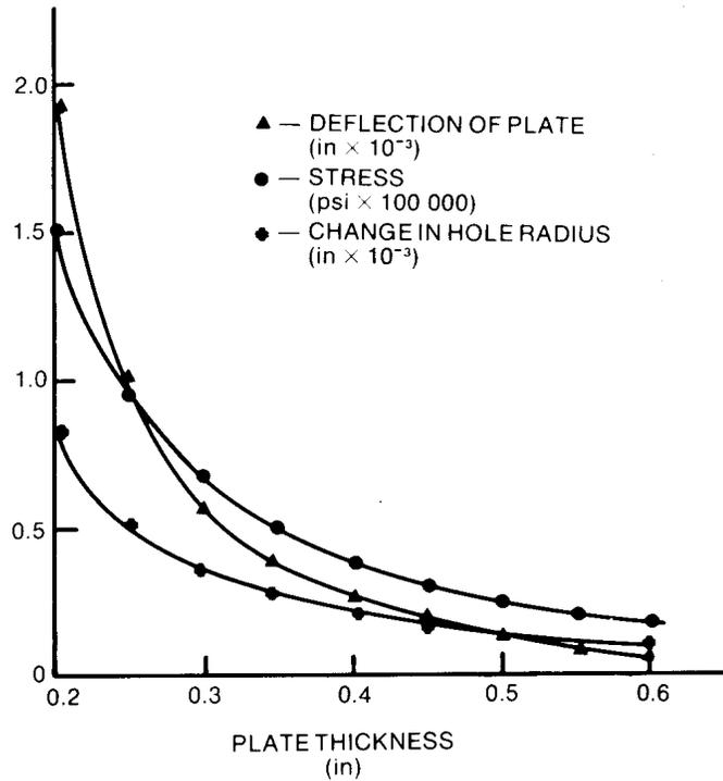
**Figure 10 - Results of plate deflection modeling for an applied pressure of 10,000 psi.**
