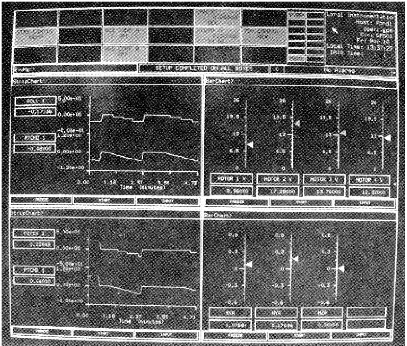
**Figure 4. Example display screen showing a snapshot of attitude control system transient behavior.**
