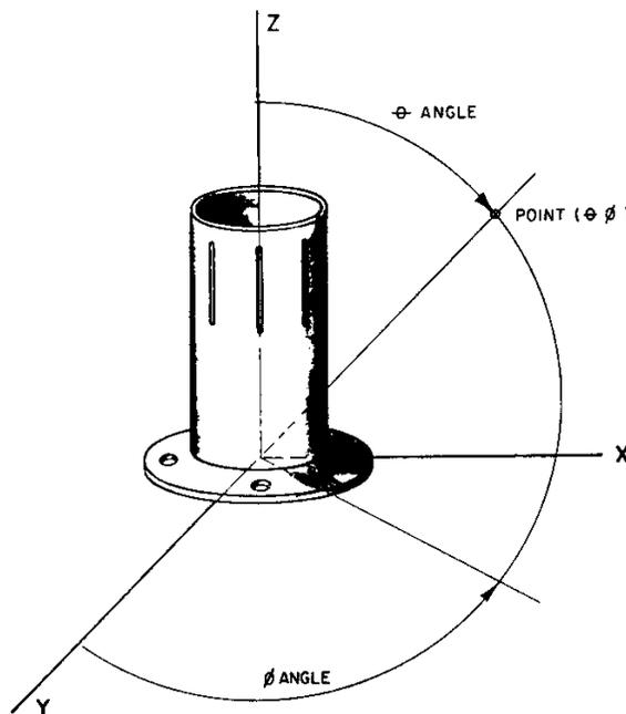
**Figure 1. Reference coordinate system.**
