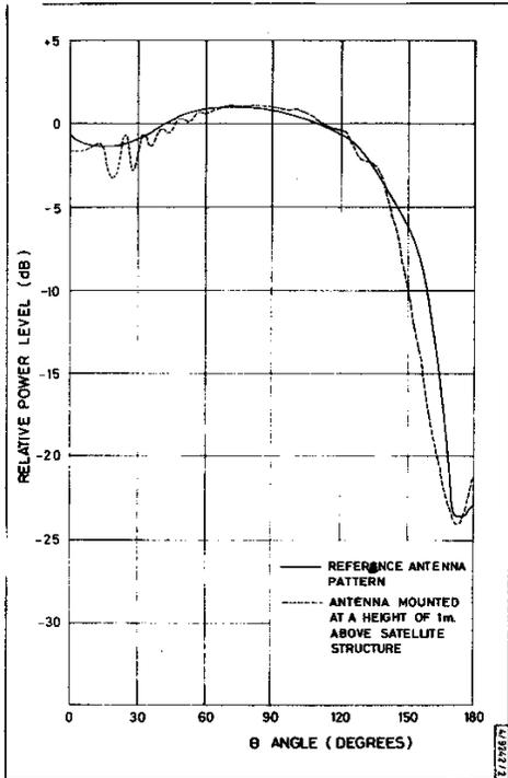
**Figure 4. Antenna pattern comparison for 'isolated' and 'satellite mounted' configuration.**
