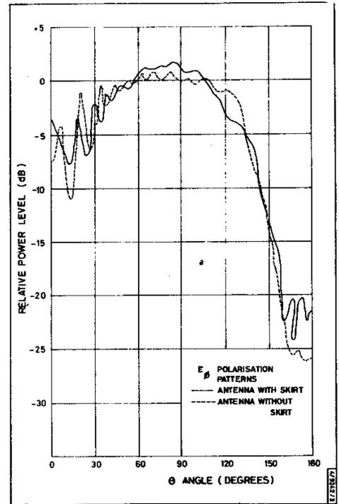
**Figure 3. Influence of the skirt on antenna radiation pattern.**
