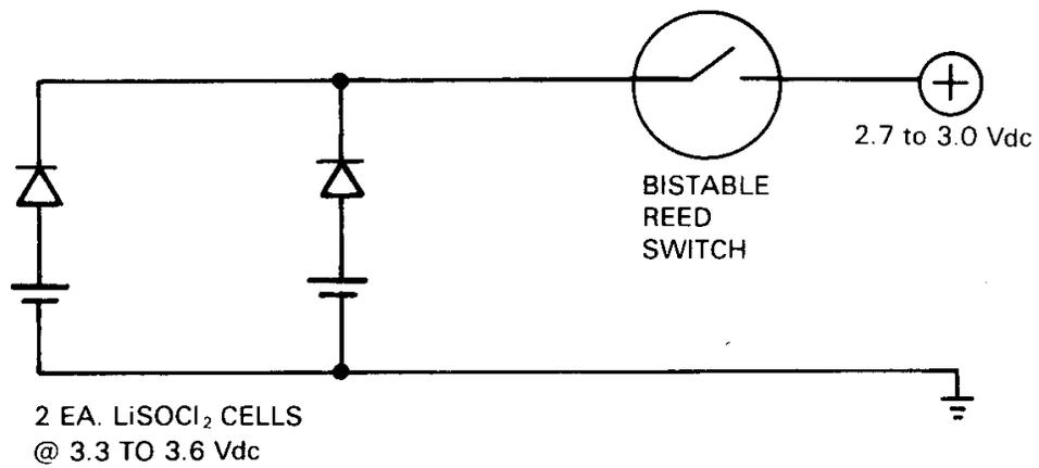
**Figure 1. 1 200 hour battery pack.**
