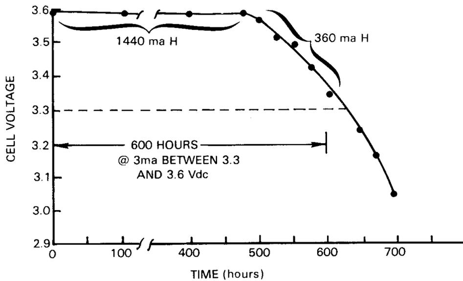
**Figure 2. AA size GTE LiSOCl<sub>2</sub> cell discharge curve under 3 ma load.**
