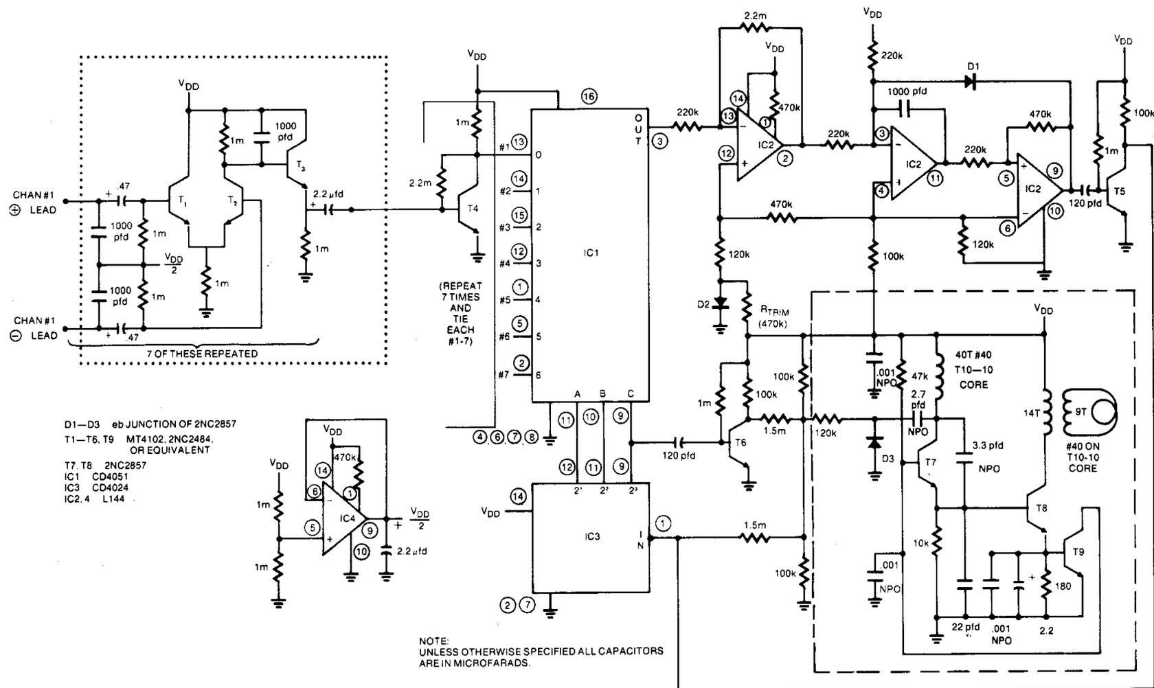
Figure 3. Seven channel hybrid telemetry transmitter.
