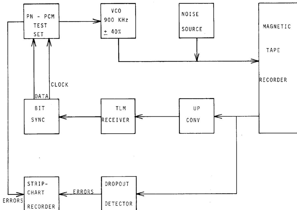
**Figure 1 - Predetection Test Configuration**
