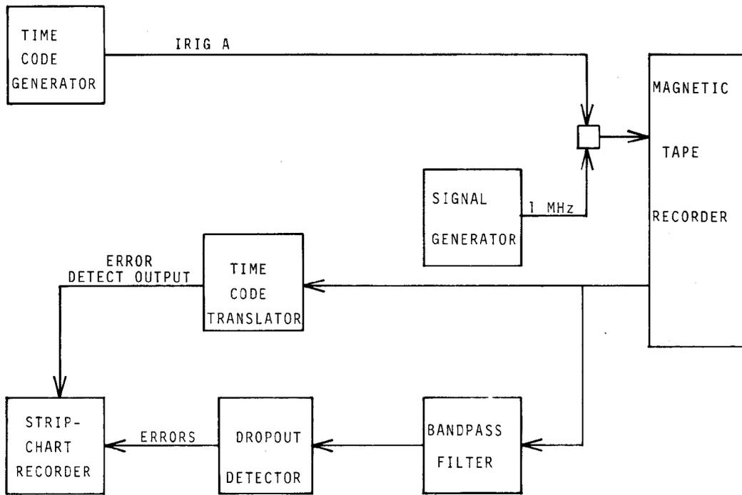
**Figure 3 - IRIG Timing Test Configuration**
