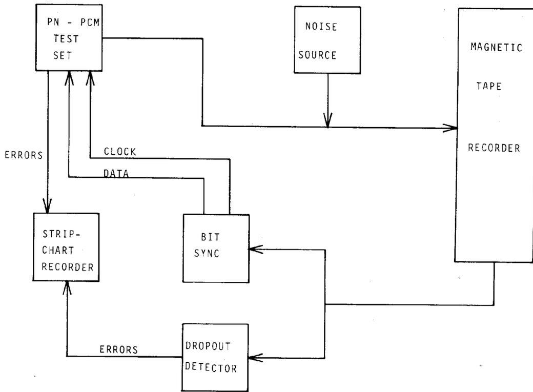
**Figure 2 - Post-detection Test Configuration**
