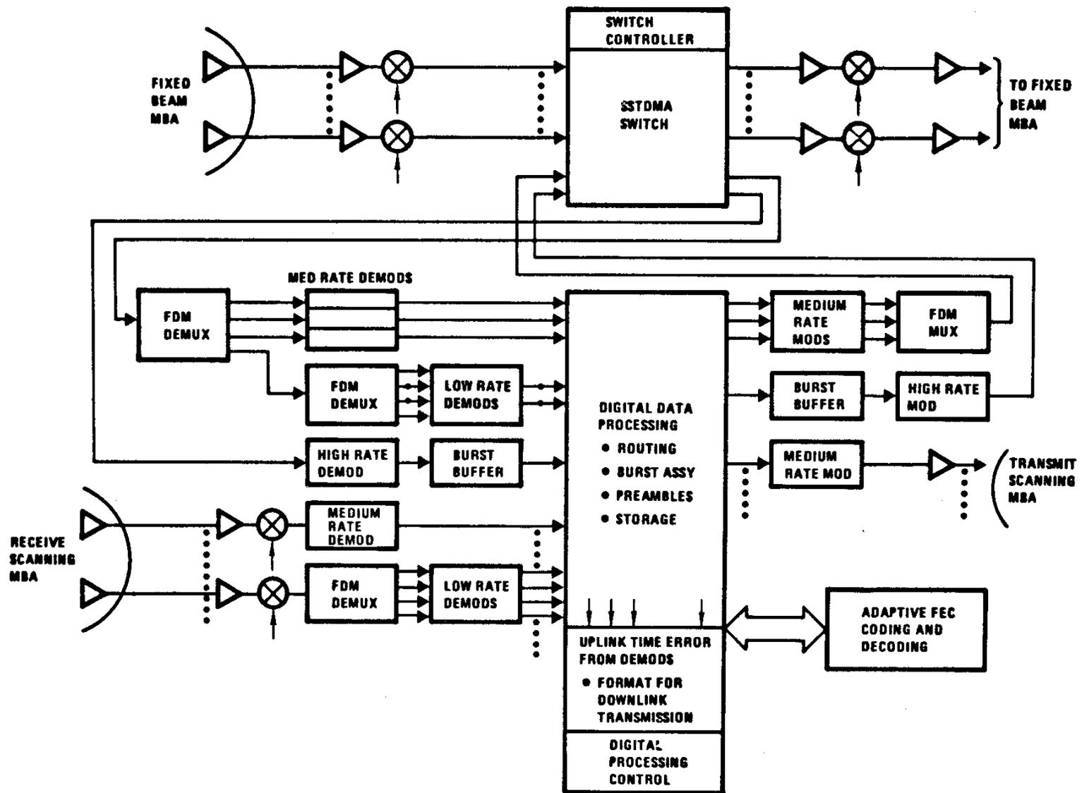
Figure 4. Satellite Communication Subsystem Block Diagram
