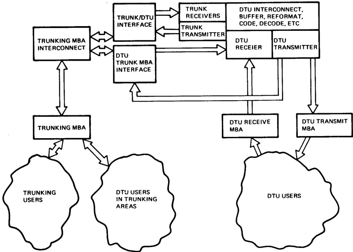
Figure 3. 20120 GHz Mixed User System Architecture
