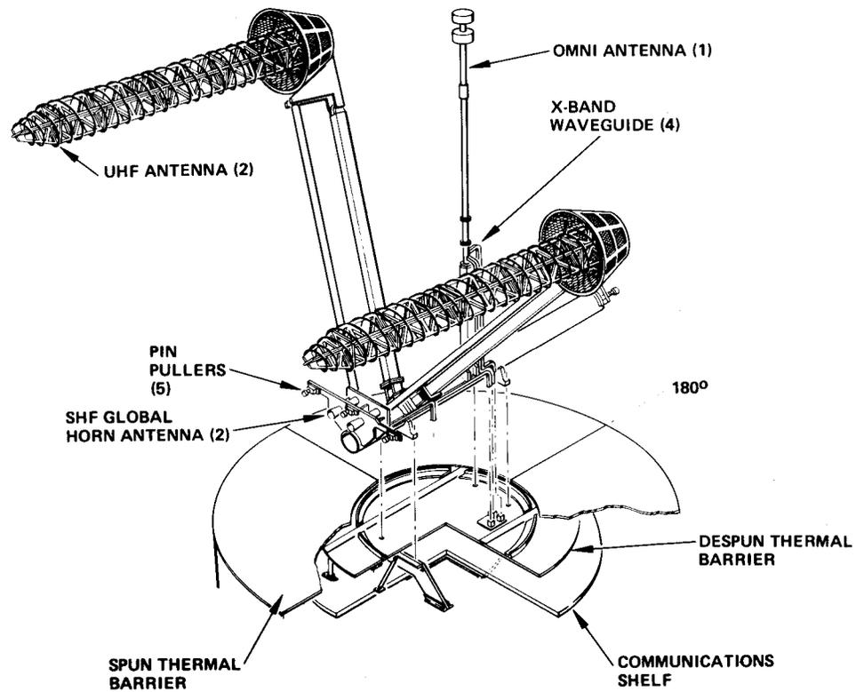
**Figure 3. LEASAT Deployed Antenna Configuration**
