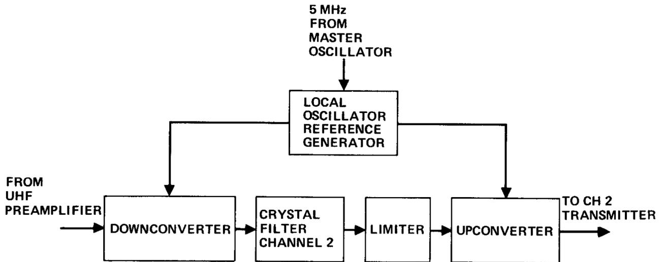
Figure 5. 500 kHz Receiver Block Diagram
