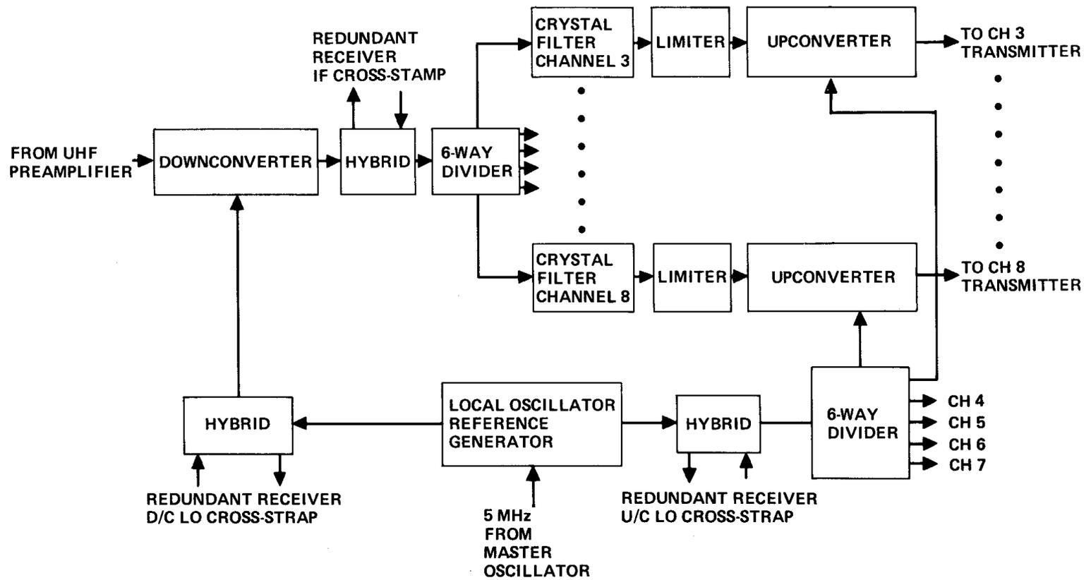
Figure 7. 25 kHz Channel Receiver
