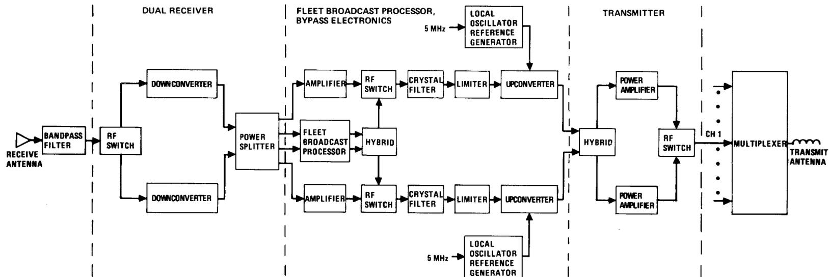
Figure 9. Fleet Broadcast Block Diagram
