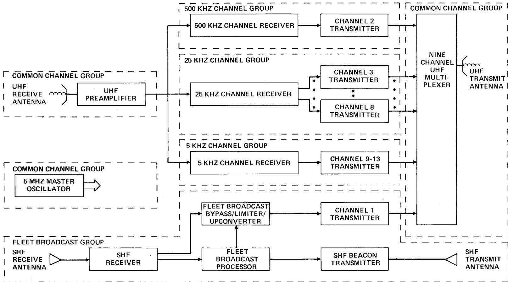
**Figure 4. Communication Subsystem Functional Groups**
