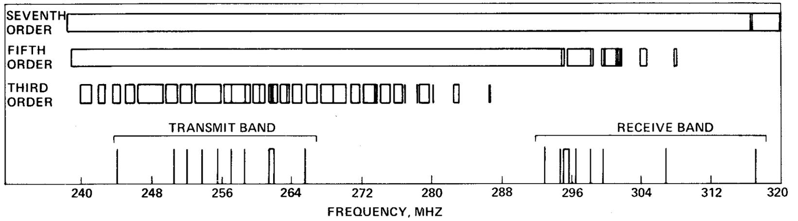
**Figure 10. LEASAT Frequency Plan Passive IM Products**
