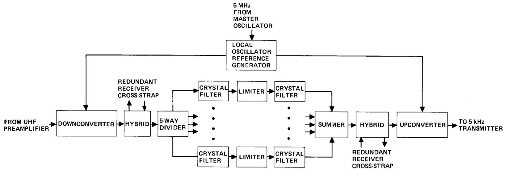
**Figure 8. 5 kHz Receiver Block Diagram**
