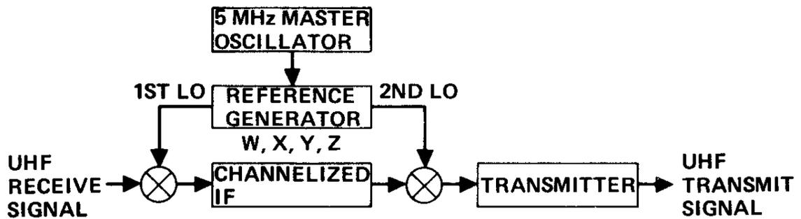
Figure 6. UHF Channel Group Typical Signal Flow
