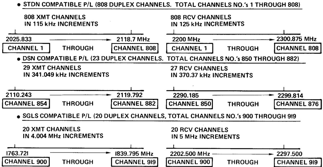
**Figure 13. Payload Interrogator RF Channels**
