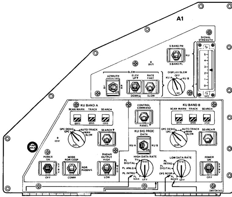
Figure 17. Ku-Band Displays and Controls
