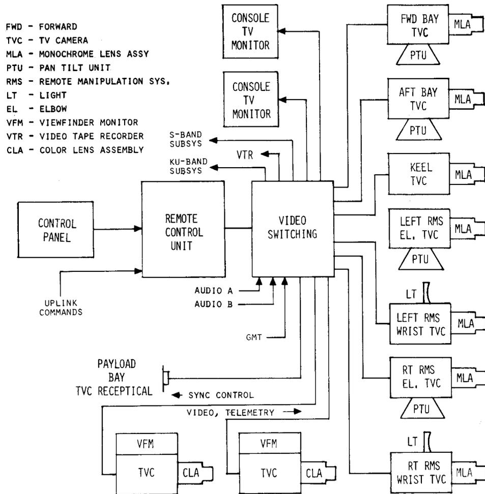
**Figure 6. Operational TV Subsystem Diagram**
