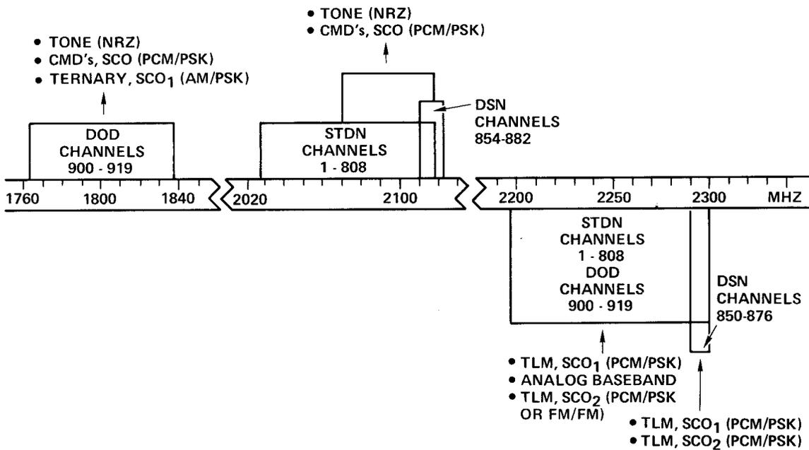
Figure 11. Payload Frequencies, Modes, and Selected Data Rates
