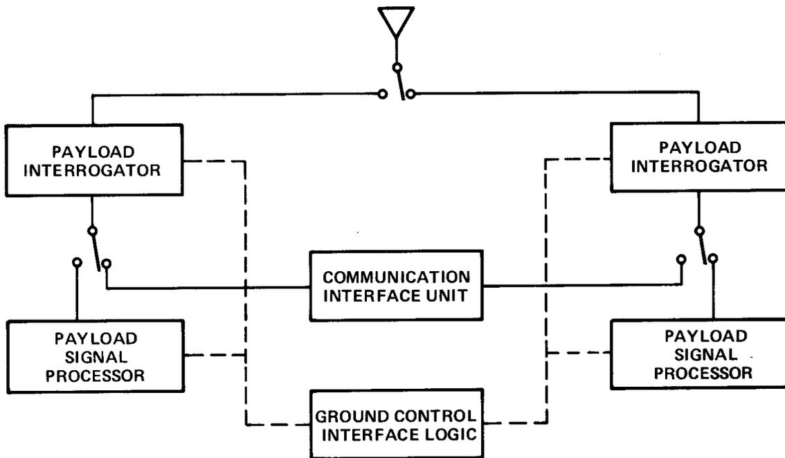
Figure 12. Payload Subsystem Block Diagram
