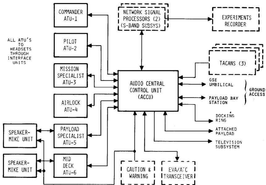
**Figure 5. Audio Distribution Subsystem Block Diagram**
