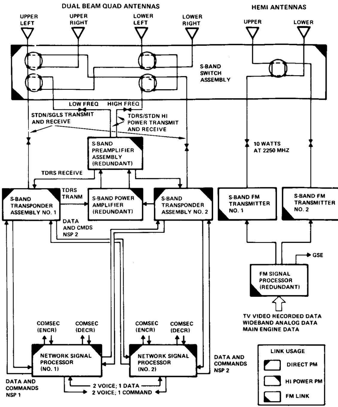
Figure 3. S-Band Subsystem Block Diagram
