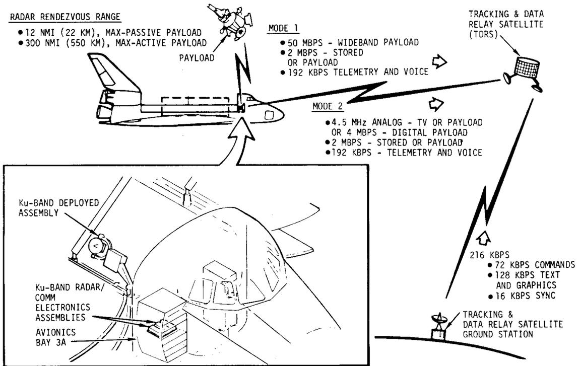
**Figure 7. Ku-Band Radar/Communication Subsystem**
