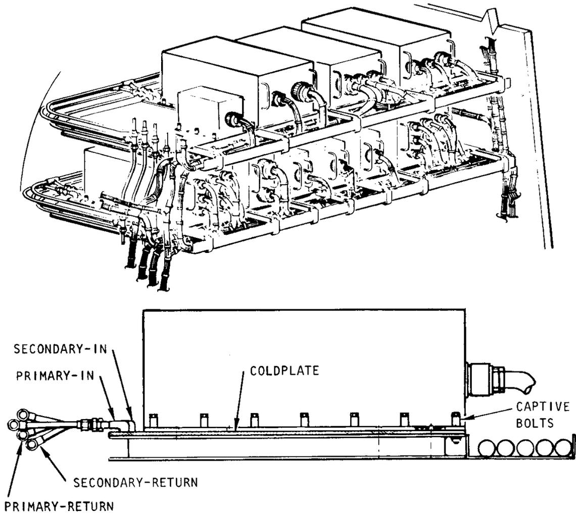
**Figure 19. Typical Avionics Installation**
