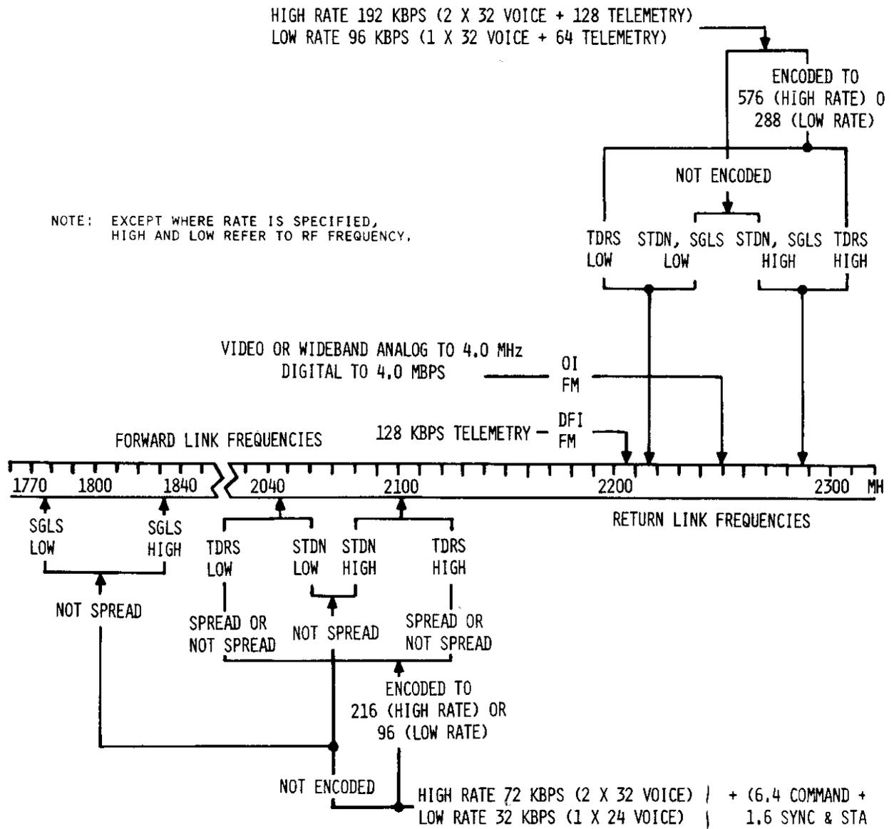
**Figure 4. S-Band Frequencies, Modes, and Data Rates**
