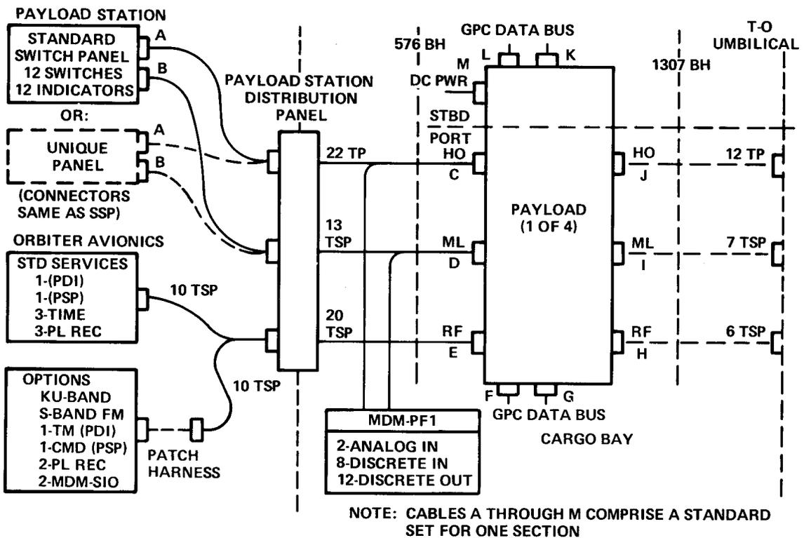
Figure 9. Standard Payload Cables for Shared Cargo Showing Services for One of Four Users
