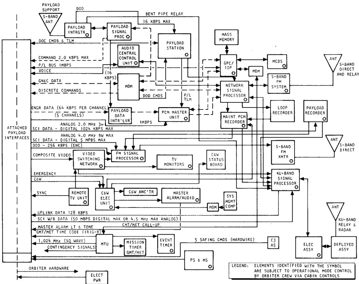
Figure 1. Standard Avionics Provisions for Payloads - Functional Diagram
