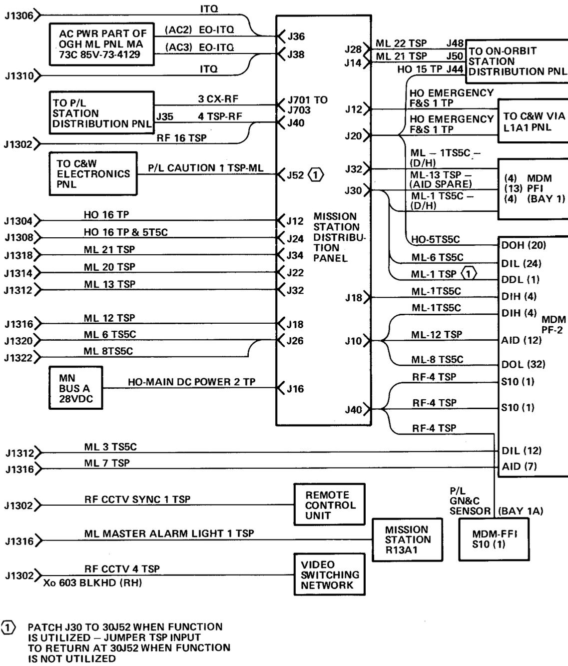
Figure 12. Nonstandard Avionics Services, Mission Station
