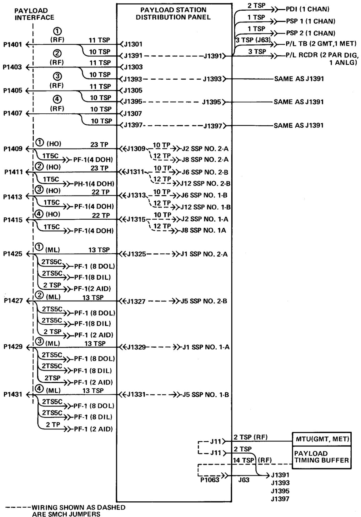
Figure 10. Standard Mixed Cargo Harnesses
