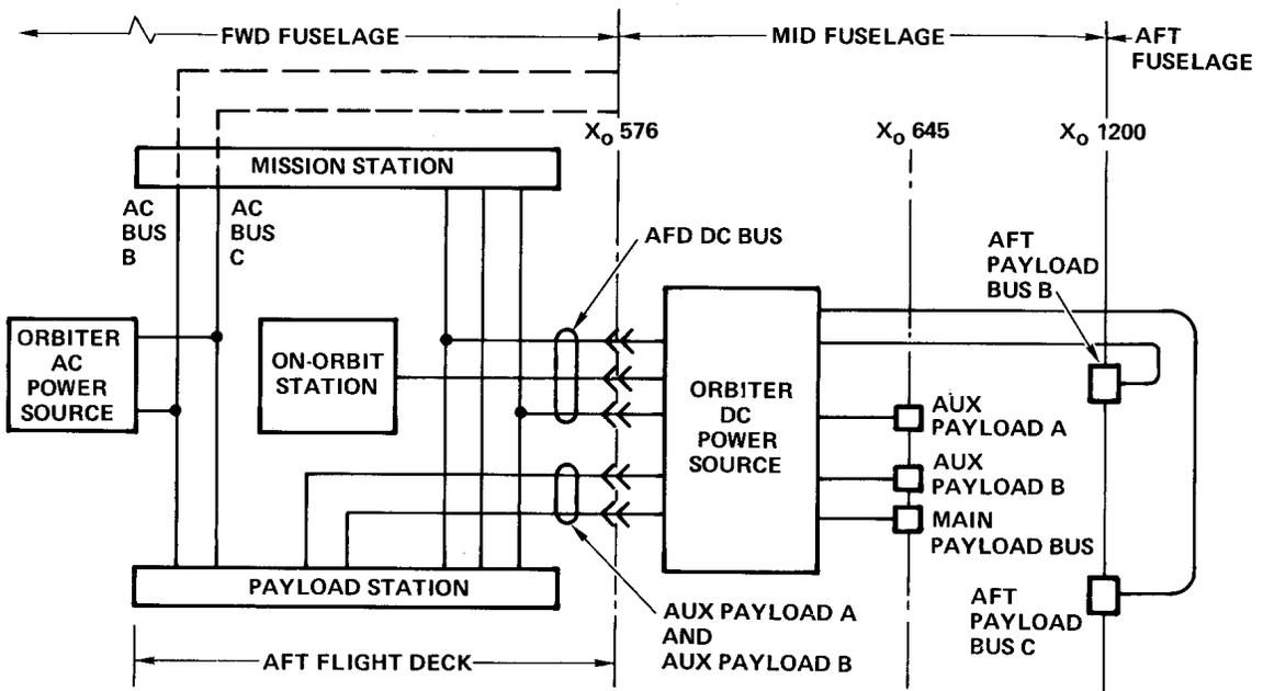
Figure 8. Payload Electrical Power Distribution System Interface
