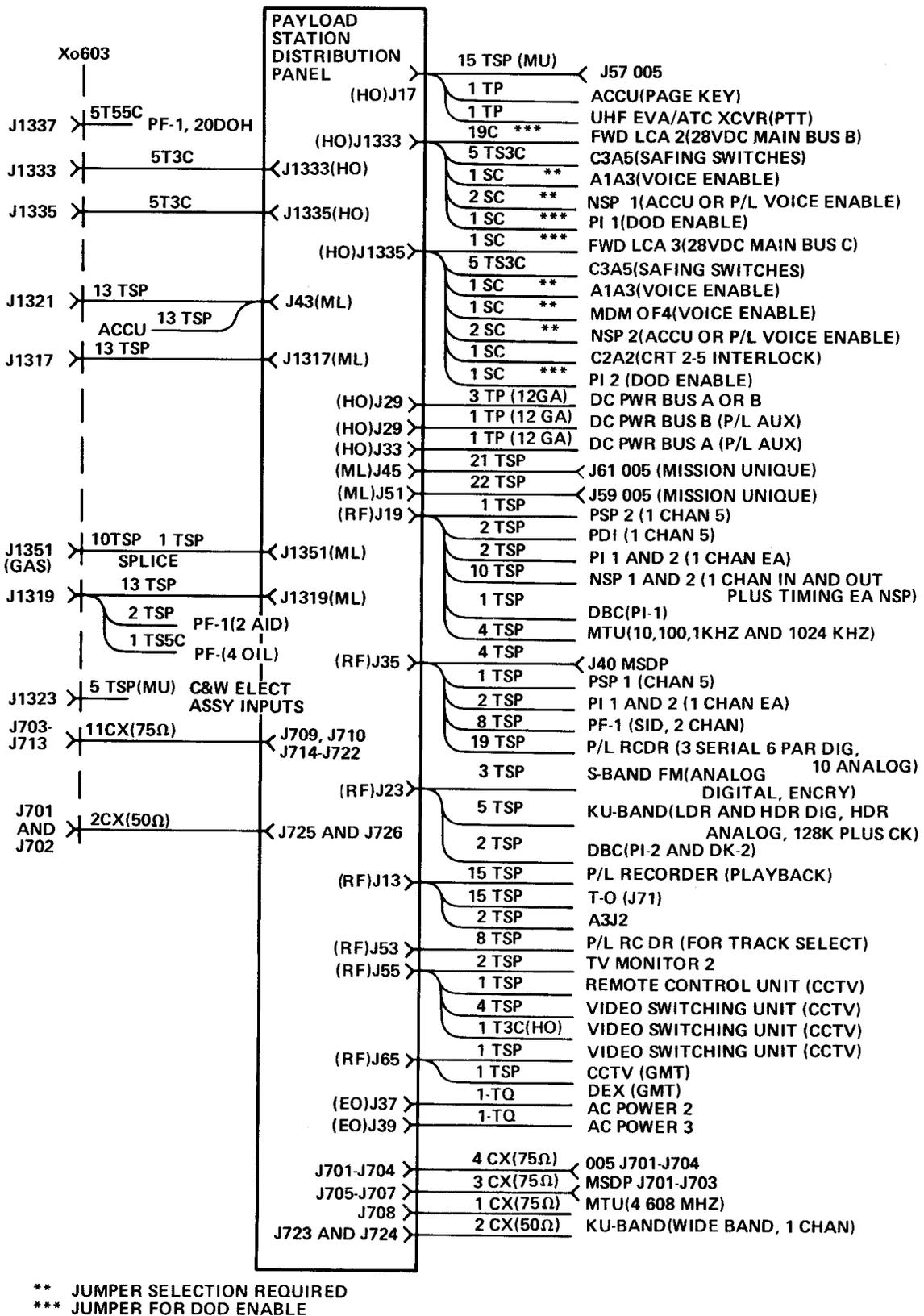
Figure 11. Nonstandard Avionics Services, Payload System
