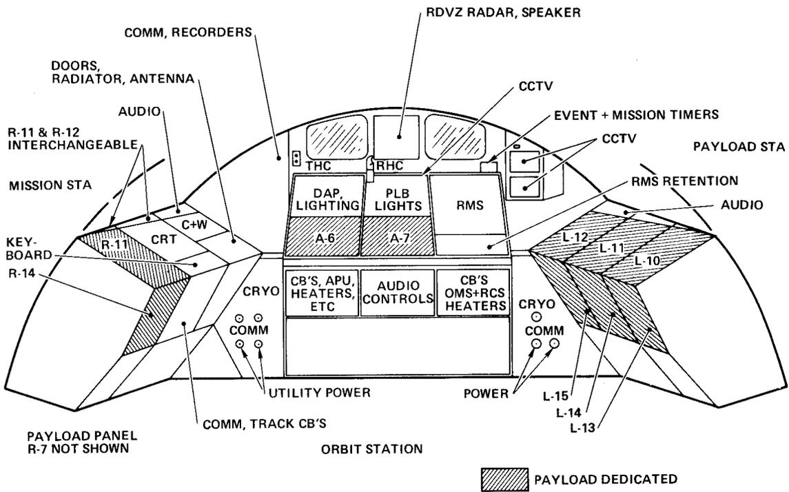
Figure 7. Aft Flight Deck
