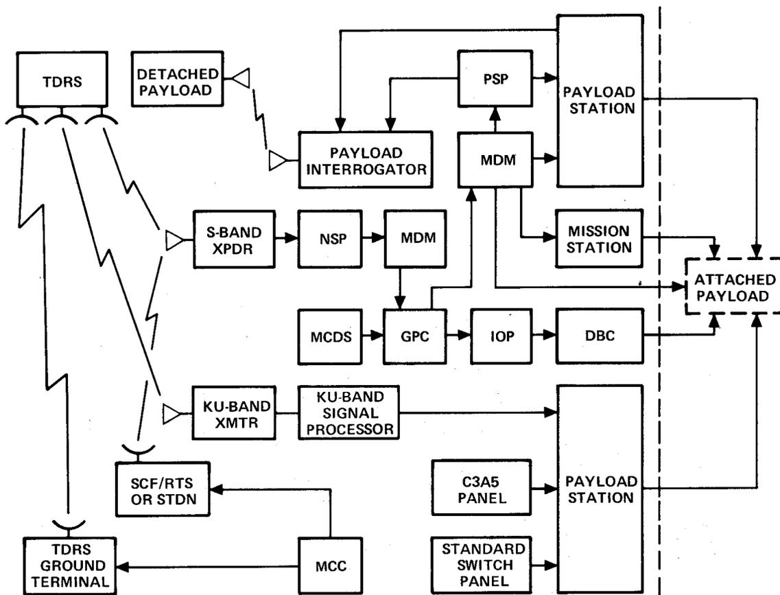
Figure 2. Payload Command System Interface Block Diagram
