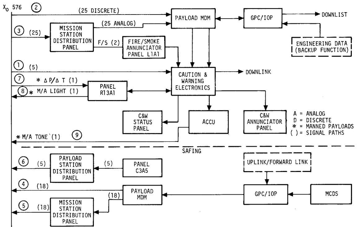
Figure 6. Payload Caution and Warning System Interface
