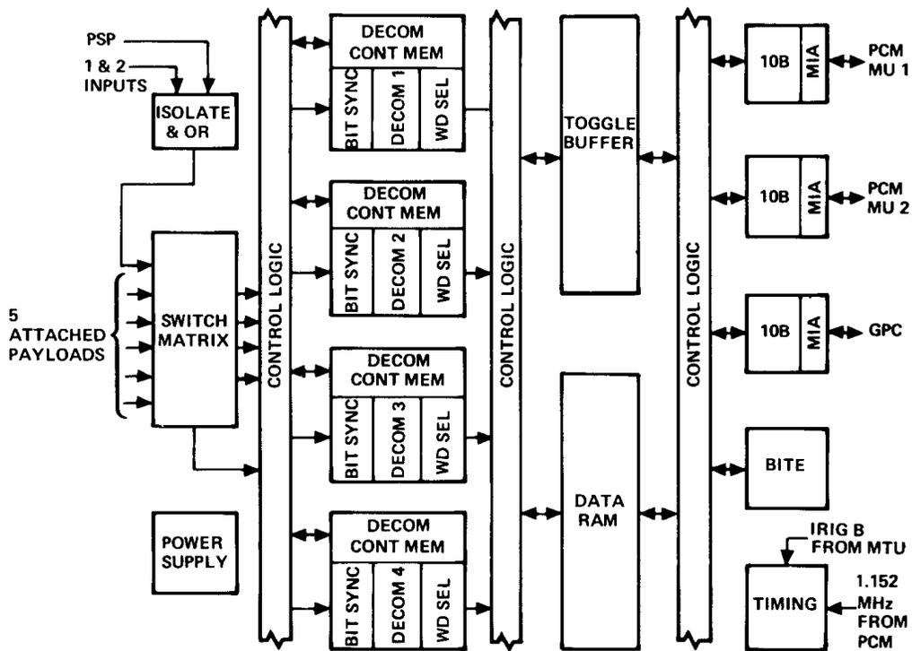
Figure 5. Payload Data Interleaver Block Diagram
