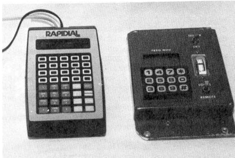
**Figure 2. Prototype Programmer with Receiver Control Elements**
