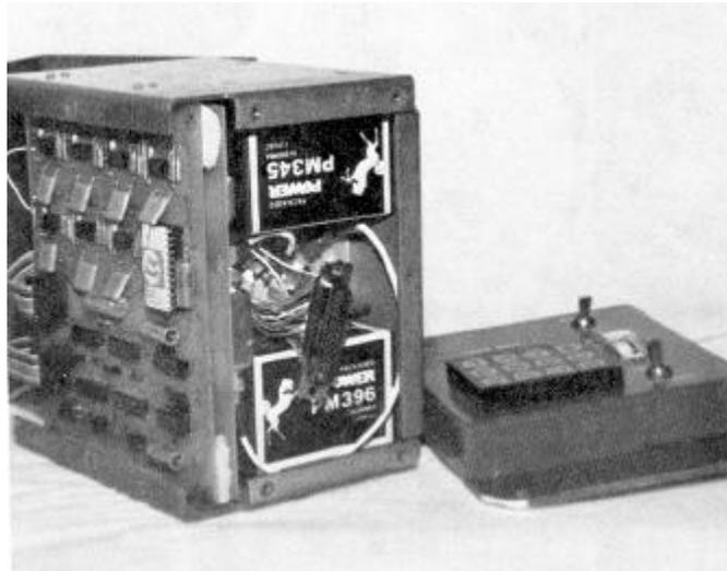
**Figure 6. TRACK model 1500-9303 TLM receiver**
