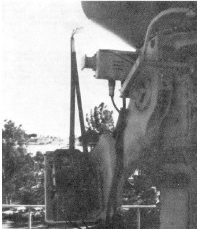
**Figure 5. WITS RF assembly mounted on AN/SPG-51 Radar**
