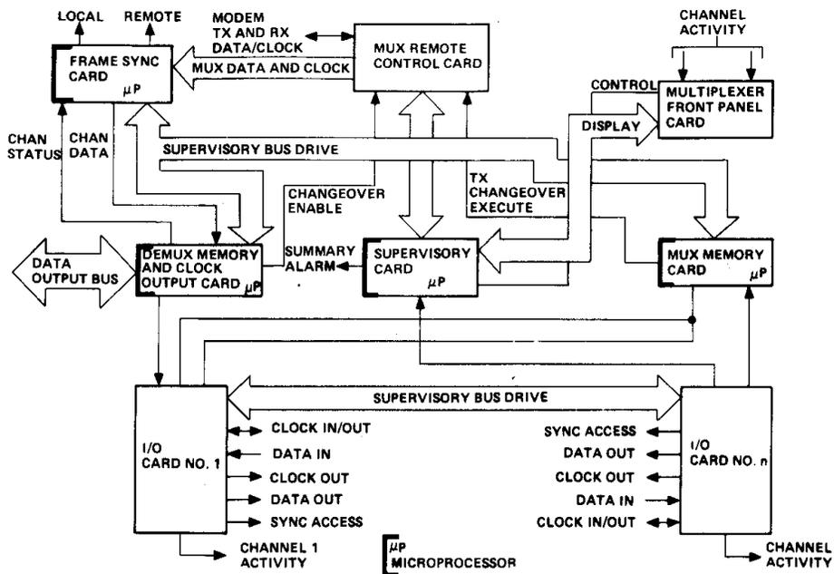
Figure 12. Ford Aerospace Smart Multiplexer Block Diagram
