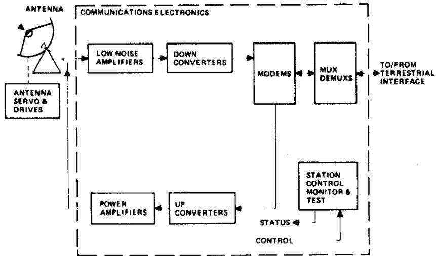
Figure 1. Earth Terminal Hardware
