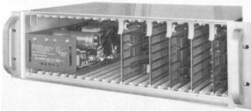
**Figure 8. DAMA Remote Station Chassis**
