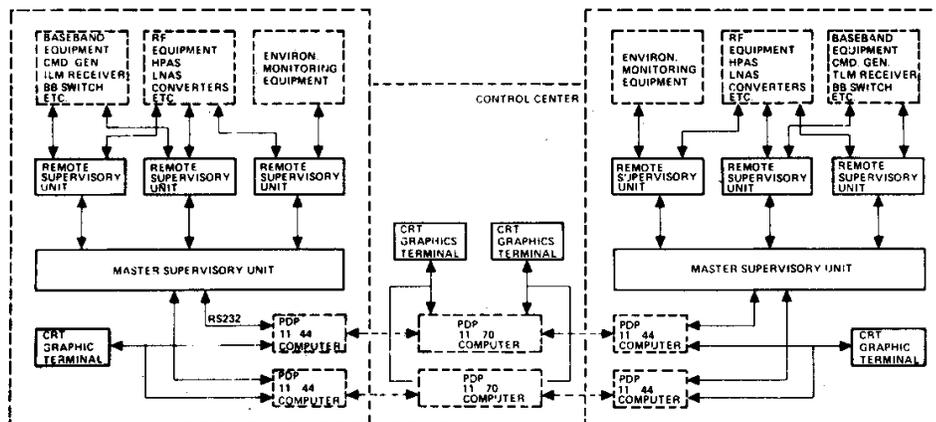
Figure 5. Supervisor Network Functional Block Diagram
