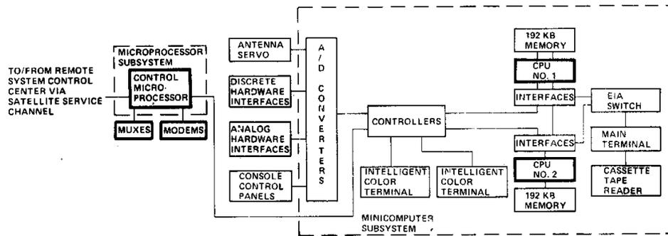
Figure 3. Earth Terminal Processor Components for Station and Network Control (FACC)
