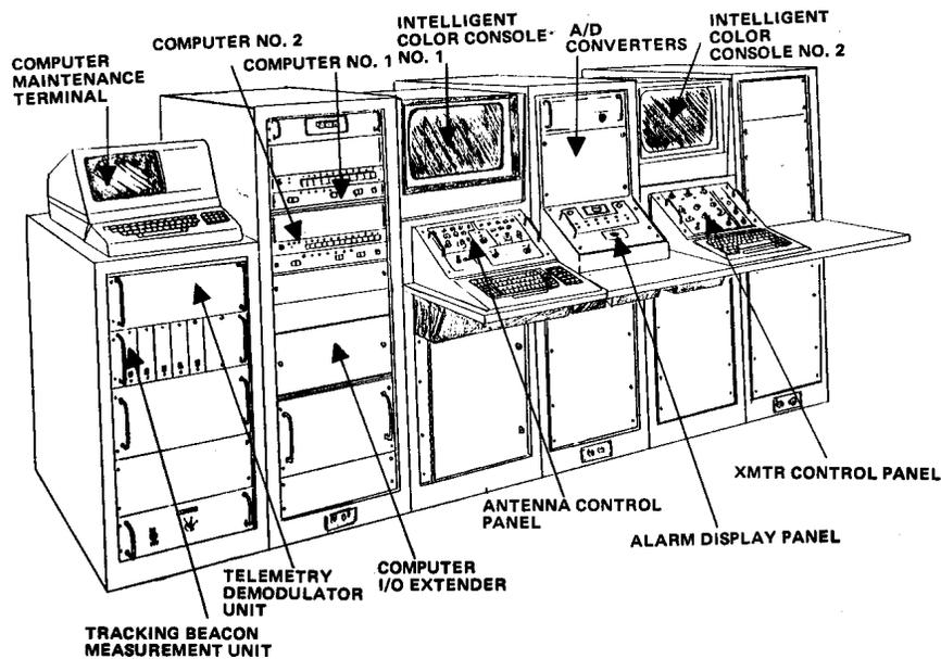
Figure 4. Computerized Earth Terminal Control Console (FACC)
