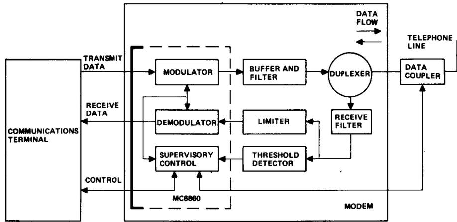
MOTOROLA'S MC68860 CHIP (DASHED BOX) PROVIDES ABOUT HALF THE FUNCTIONS NECESSARY TO FORM A SIMPLE, LOW-SPEED, FSK MODEM FOR USE WITH THE FIRM'S M6800 MICROPROCESSOR. THE MC68860 TRANSMITS 8-STEP, SYNTHESIZED SINE WAVES AND USES FILTERS ONLY ON RECEIVING.
