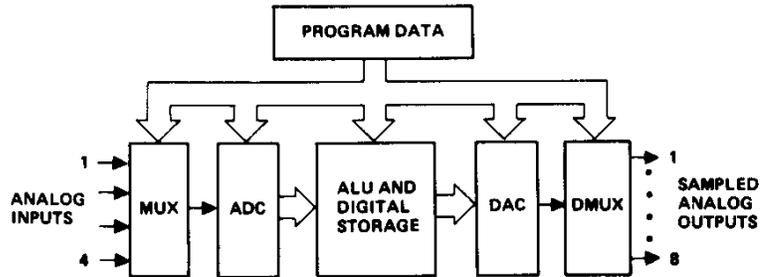
Figure 11. 2920 Signal Processor Functional Block Diagram
