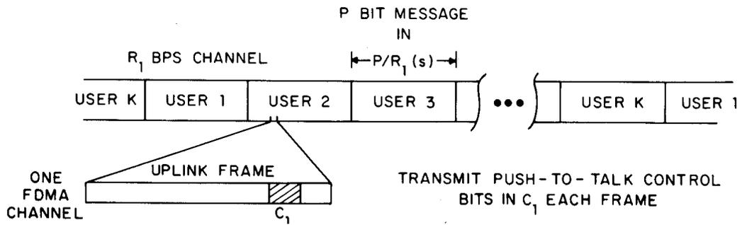
**Figure 6. The usage of a  $C_1$  control channel to transmit push-to-talk control messages to the central controller from users 1 to K in turn.**
