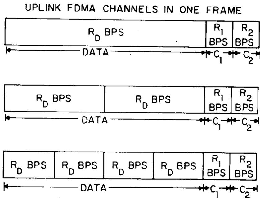
**Figure 5. Uplink transmission modes for transmitting 1,2, or 4 data streams. The  $C_1$  and  $C_2$  control transmissions do not change.**
