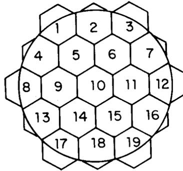
**Figure 2. Earth field-of-view covered by N=19 hexagonally packed areas.**
