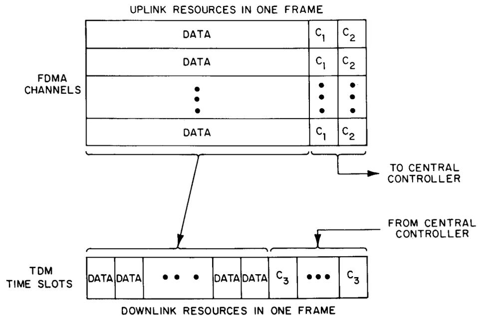
**Figure 3. Partitioning uplink and downlink resources to form data and control channels. The control flow to and from a central controller is shown.**
