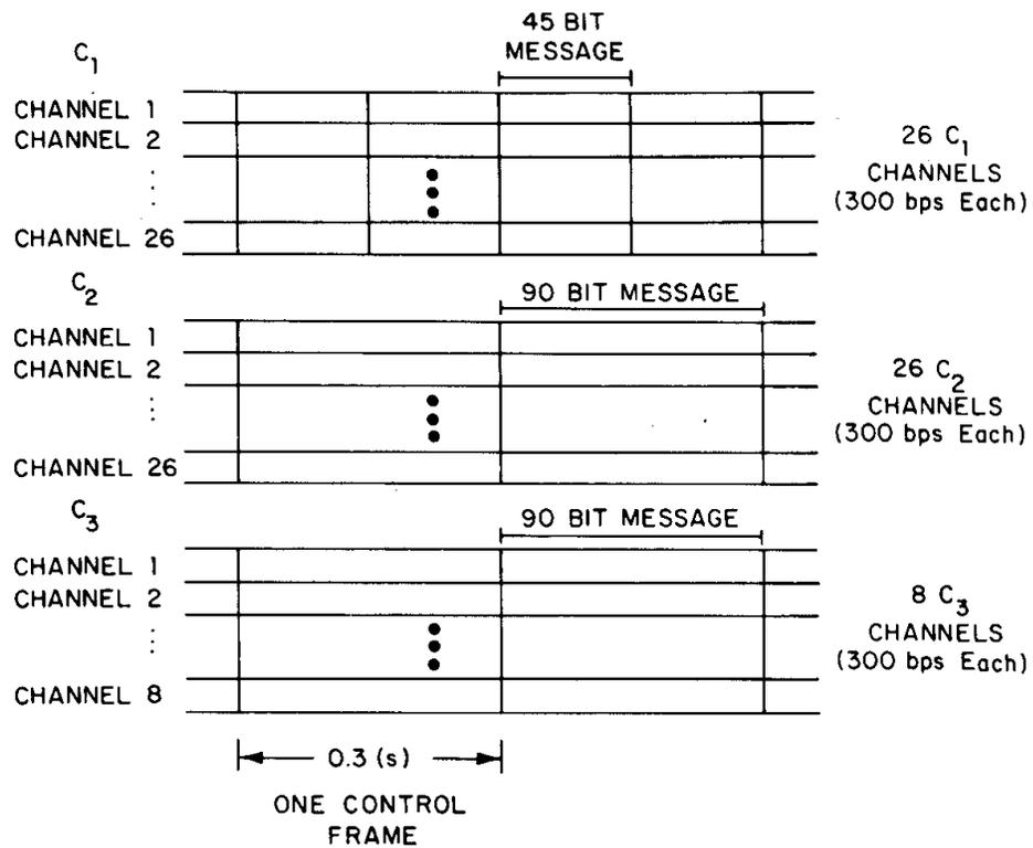
**Figure 7. Example control frame for 300 bps control channels with 45 or 90 bit control messages.**
