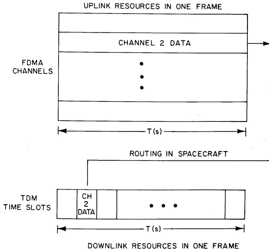
**Figure 1. The formation of channels using FDMA uplink resources and TDM downlink resources.**
