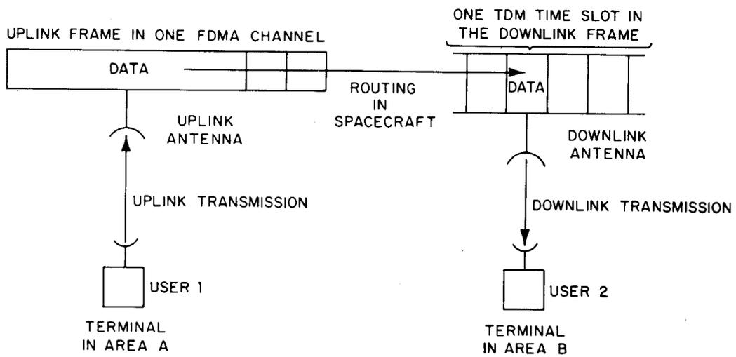
**Figure 4. Operation of a half-duplex call with the transmission path from user 1 to user 2.**
