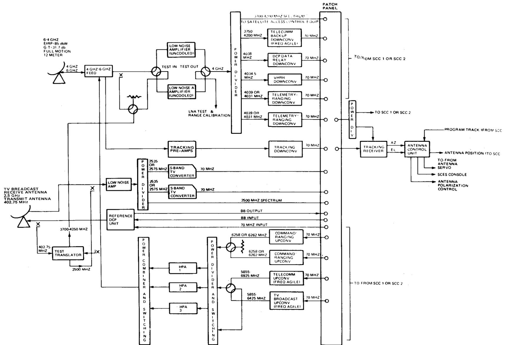
Figure 6. Satellite Control Earth Station (SCES) Functional Block Diagram
