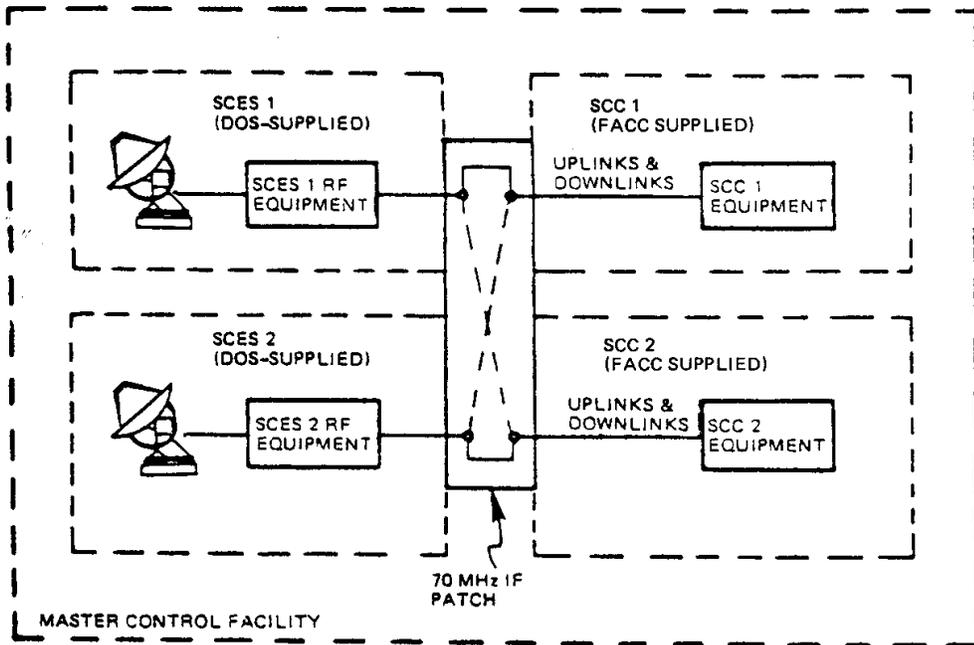
Figure 2. Master Control Facility (MCF) Elements
