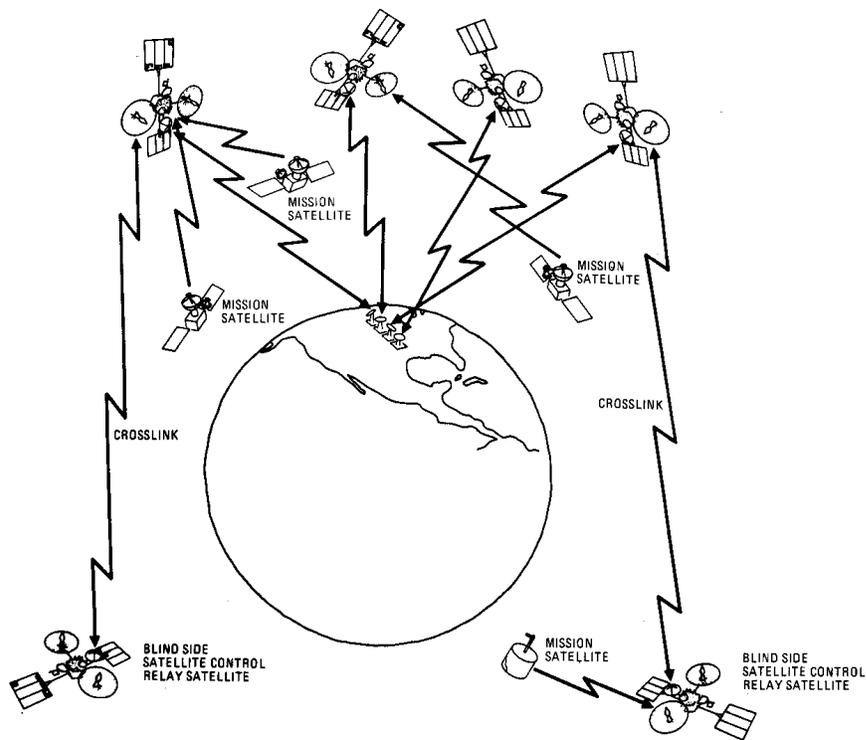
**ILLUSTRATION OF DEDICATED SATELLITE CONTROL SATELLITE SYSTEM INCLUDING CROSSLINKING**
