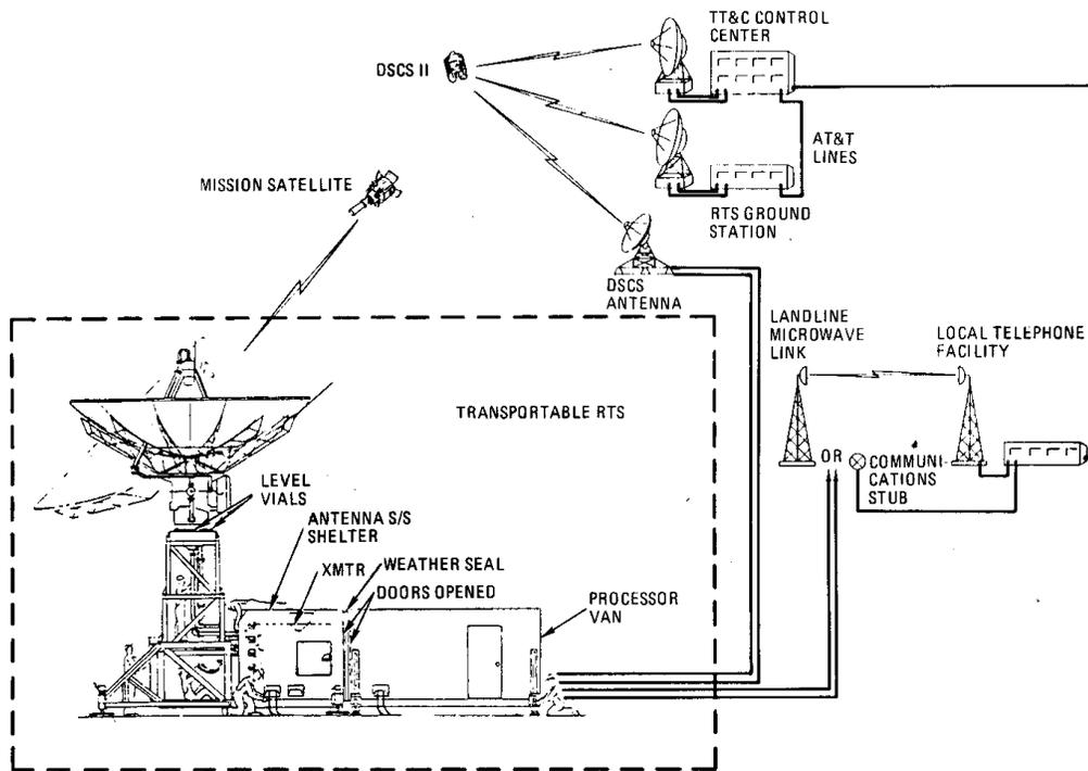
**CONCEPTUAL DEPLOYMENT OF A TRANSPORTABLE/MOBILE RTS INTO THE AFSCF NETWORK**
