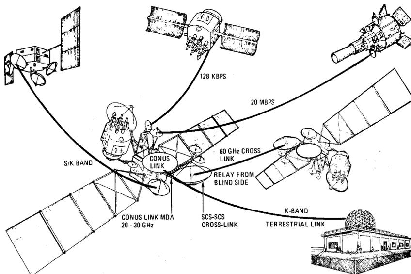
**CONCEPTUAL "ADD ON" SATELLITE CONTROL PACKAGE ON A GPS HOST SATELLITE**
