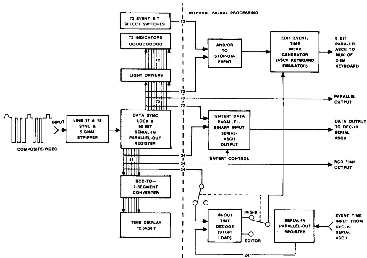
Figure 4. VIDRU Functional Block Diagram
