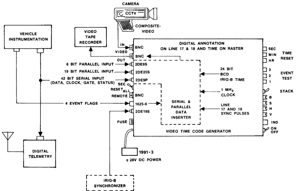
Figure 3. VTC/DDI Deployment Block Diagram
