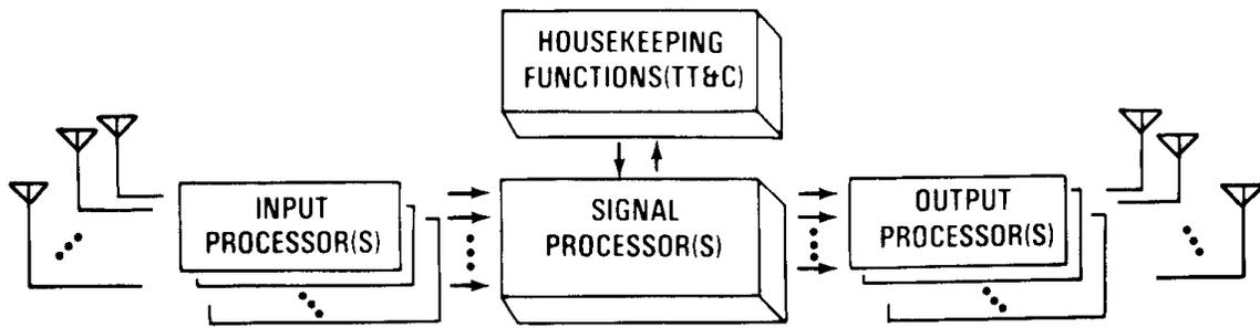
**FIGURE 3, GENERIC FUTURE MILSATCOM SATELLITE ARCHITECTURE WITH HOUSEKEEPING FUNCTIONS**
