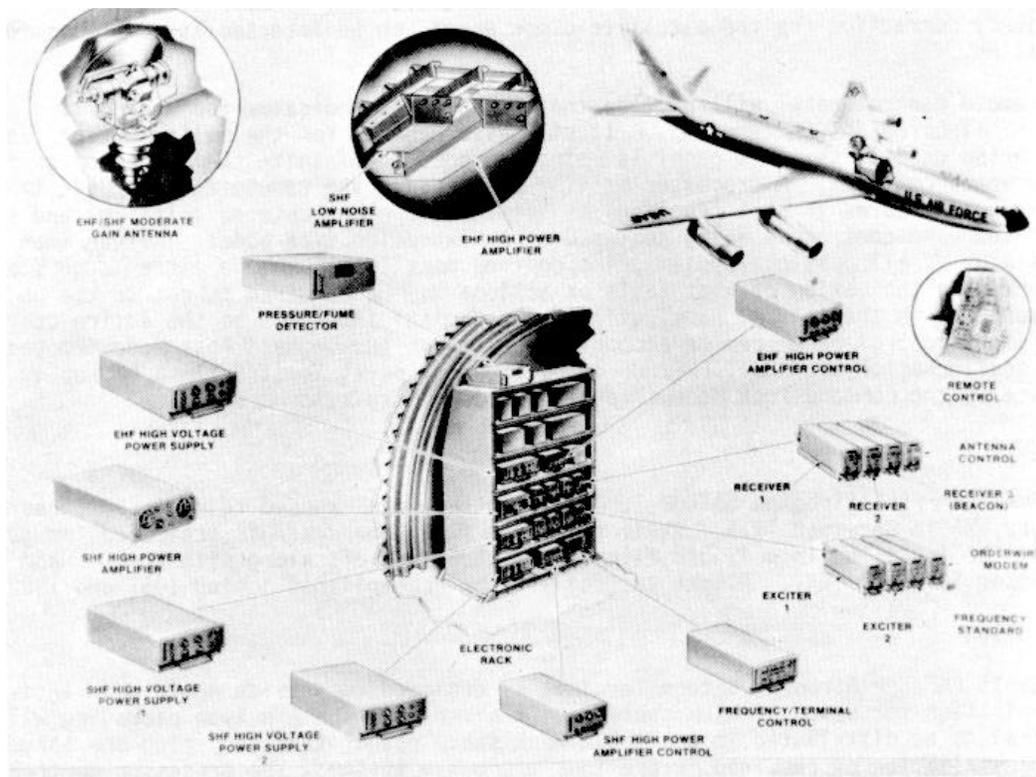
**FIGURE 1 SMALL EHF/SHF AIRBORNE SATCOM TERMINAL**
