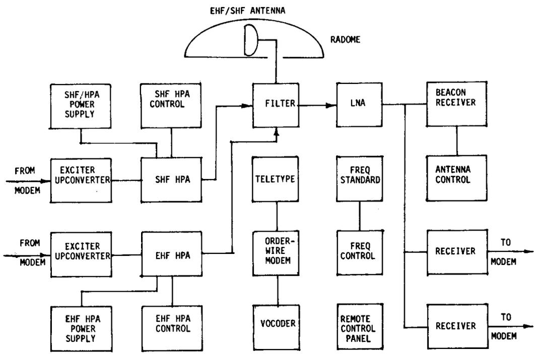
**FIGURE 2 SMALL EHF/SHF AIRBORNE SATCOM TERMINAL BLOCK DIAGRAM**
