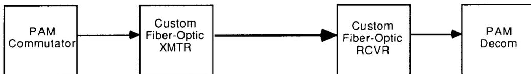
**Figure 5. A PAM System Using an Analog Fiber-Optic System That Conserves the DC Level.**
