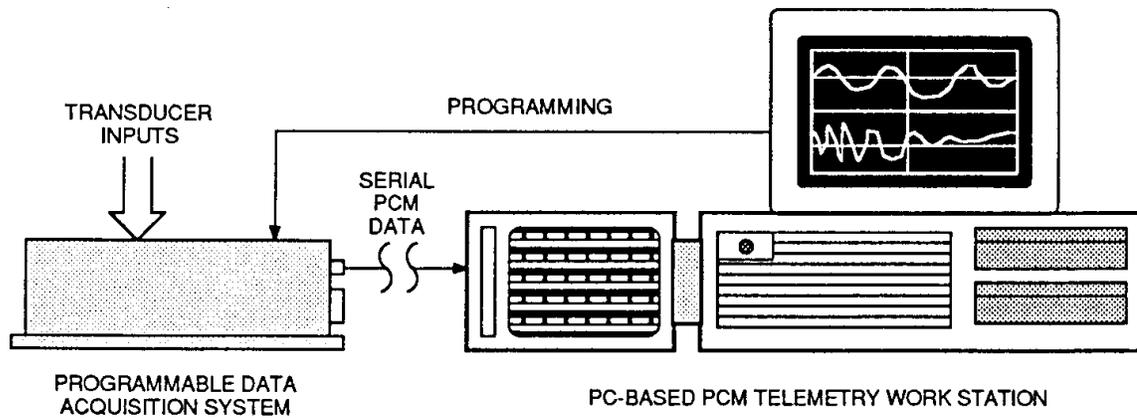
**Figure 1. An End-to-End Programmable PCM Telemetry System**
