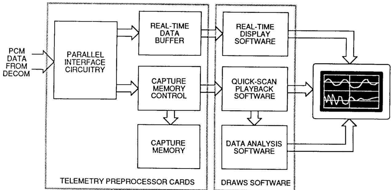
**Figure 3. DRAWS PCM Telemetry Work Station**
