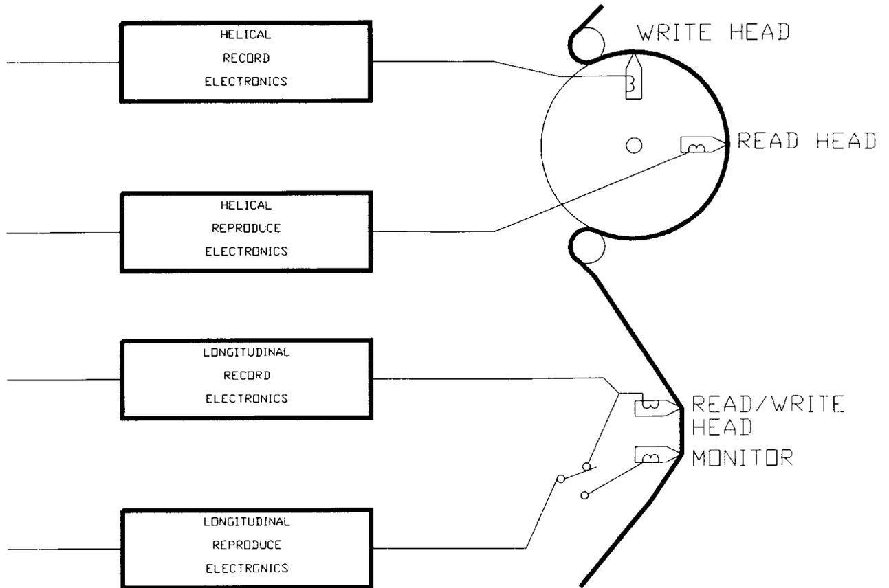
**Figure 1. 19mm Recorder Tape Path**
