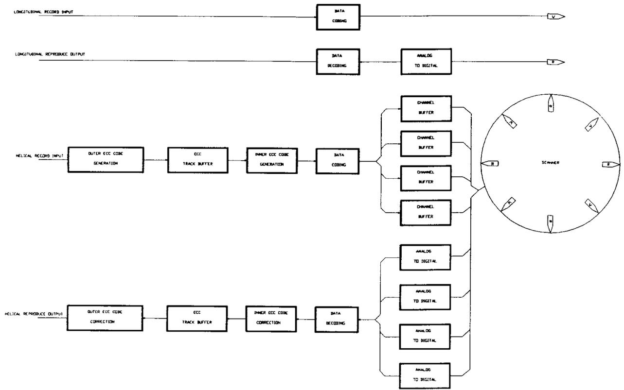
Figure 2. 19mm Recorder Block Diagram
