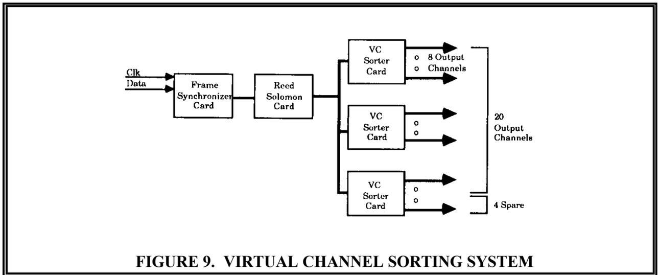
multiple VC Sorter Cards. Each VC Sorter Card can sort VCDU's to up to 8 output channels. Up to 8 Sorter Cards could be used in the VCSS for a maximum of 64 output channels. Each VC Sorter Card output represents the set of VCDU's from a space-ground link that are bound for a particular FLD. Three VC Sorter Cards could satisfy the requirement of the DIF RLP for 20 channels, with 4 channels left as spares.
