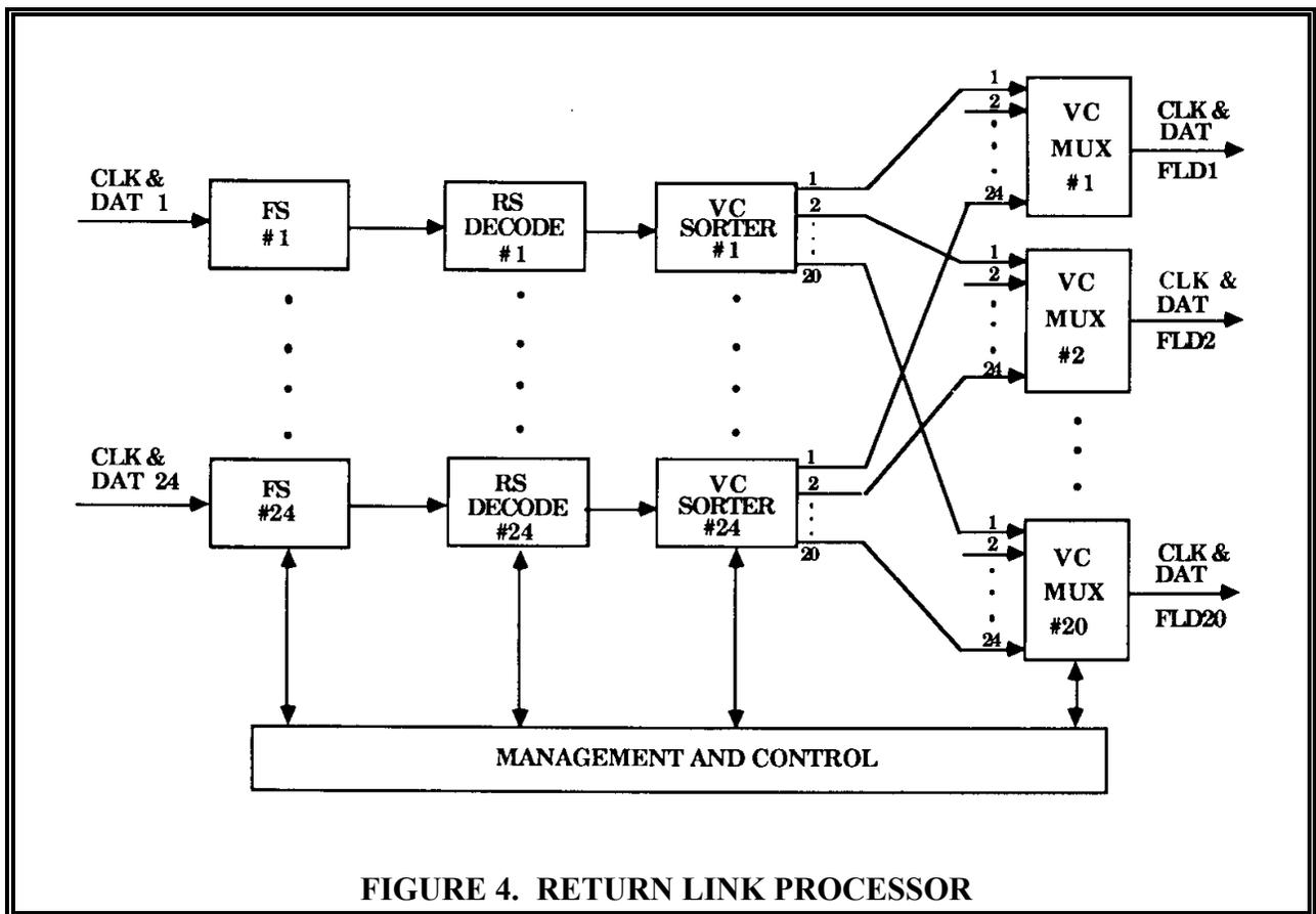
**FIGURE 4. RETURN LINK PROCESSOR**
