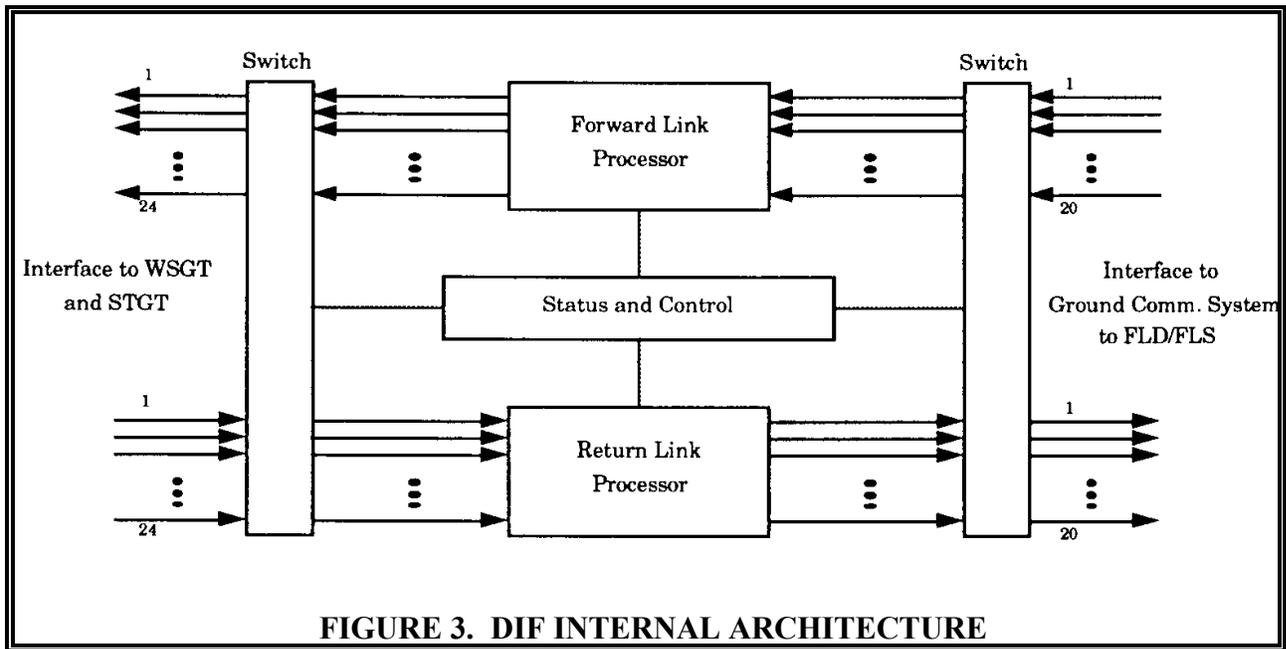
system side also performs two functions. On the return link, it selects the ground communication interface to the FLD and can select another in the case of a failure. On the forward link, the switch selects the element of the Forward Link Processor (FLP) that will serve a particular First Level Source (FLS).
