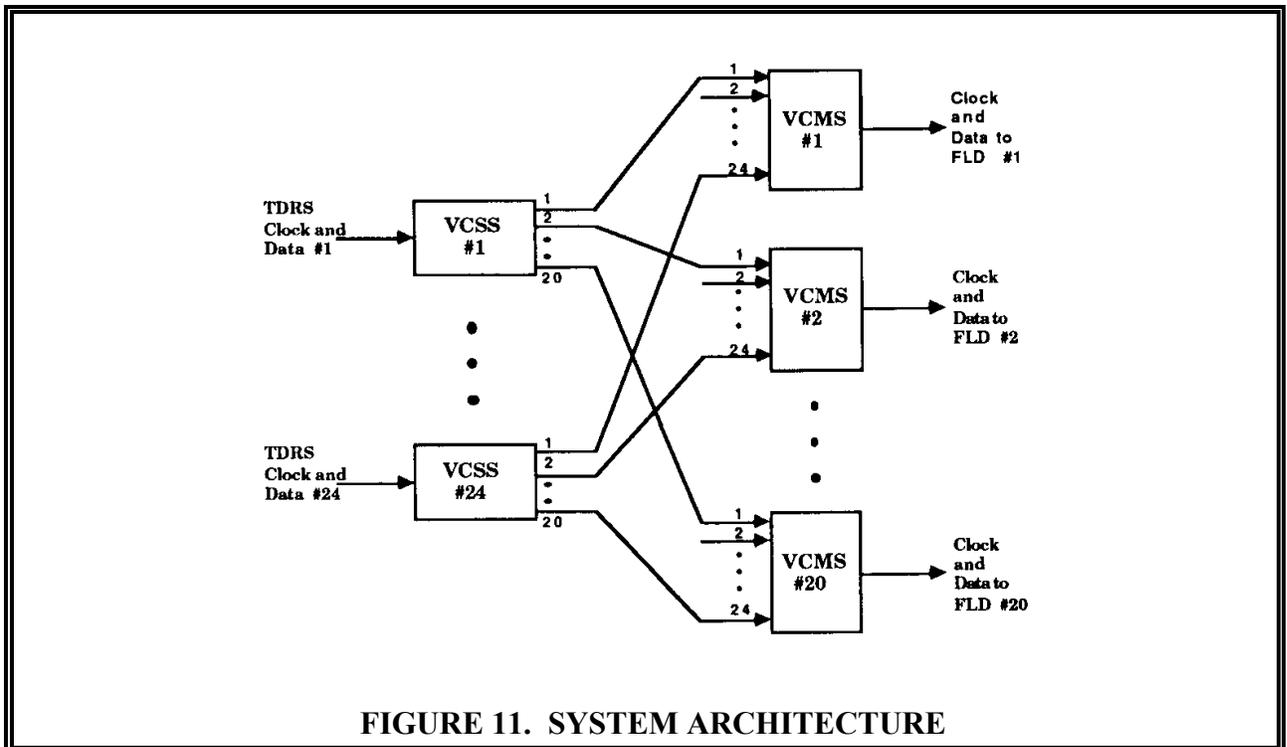
Therefore, the core functions of the DIF Return Link Processor could be implemented using 24 VCSS's and 20 VCMS's. Each of these systems is contained in one 19 inch VME card cage. Four of these card cages fit into one six foot rack. Therefore, an implementation would include six Sorting Racks, each containing four VCSS's, and five Multiplexing Racks, each containing four VCMS's. The fully integrated system would be housed in a total of eleven six foot racks (figure 12).
