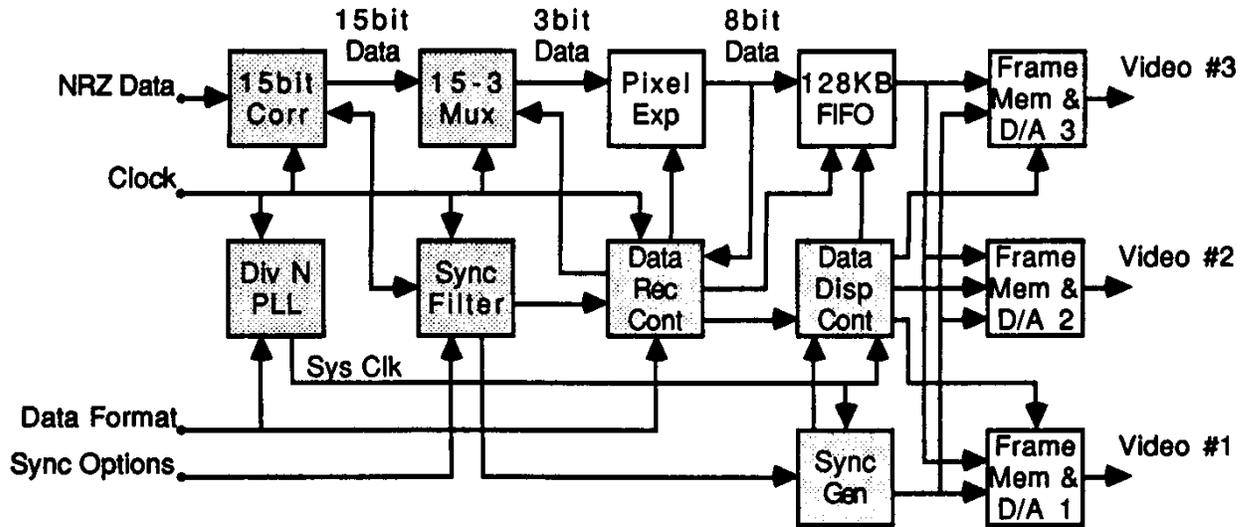
**Figure 4: Simplified Digital Video Decoder Block Diagram**
