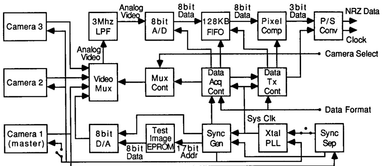
**Figure 2: Simplified Digital Video Encoder Block Diagram**
