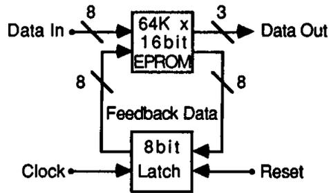
**Figure 3: Pixel Compressor**
