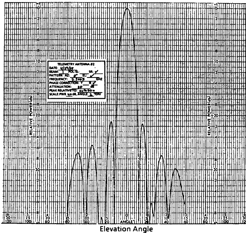
b). Elevation Plane Pattern (Boresight).
