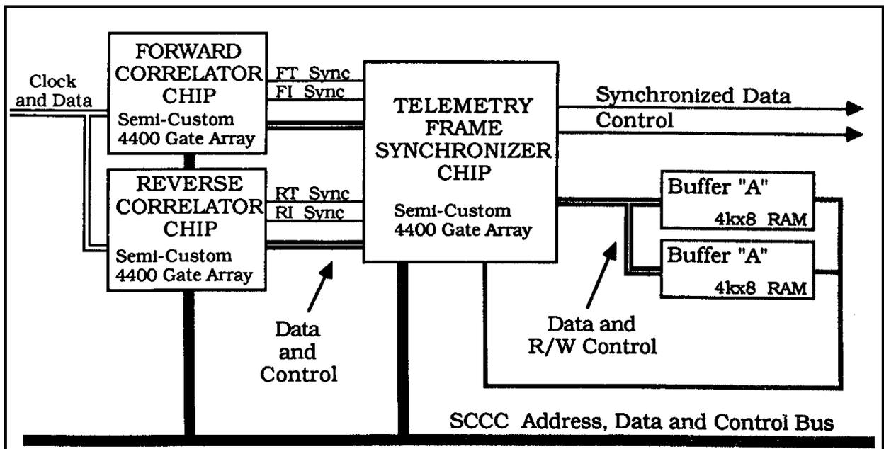
Figure 3 - Telemetry Frame Synchronizer Chip Set
