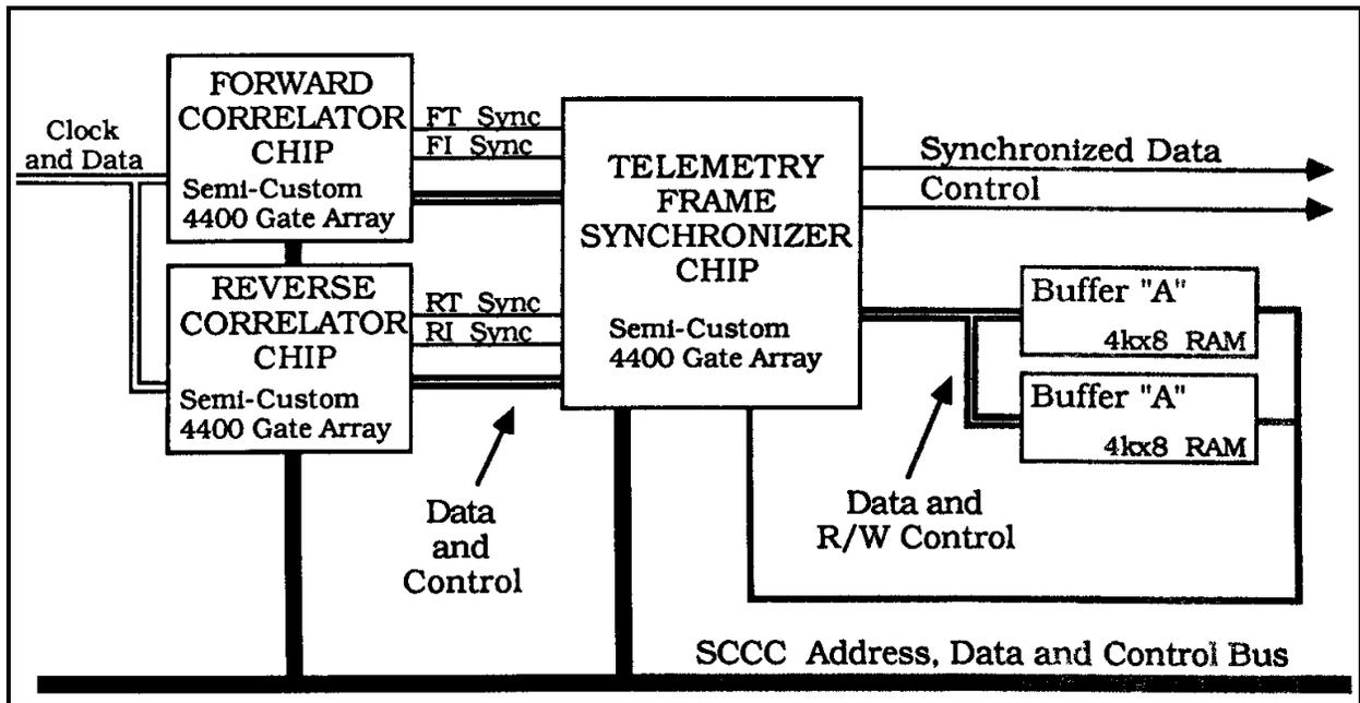
Figure 2 - NASCOM Block Processor Chip Set
