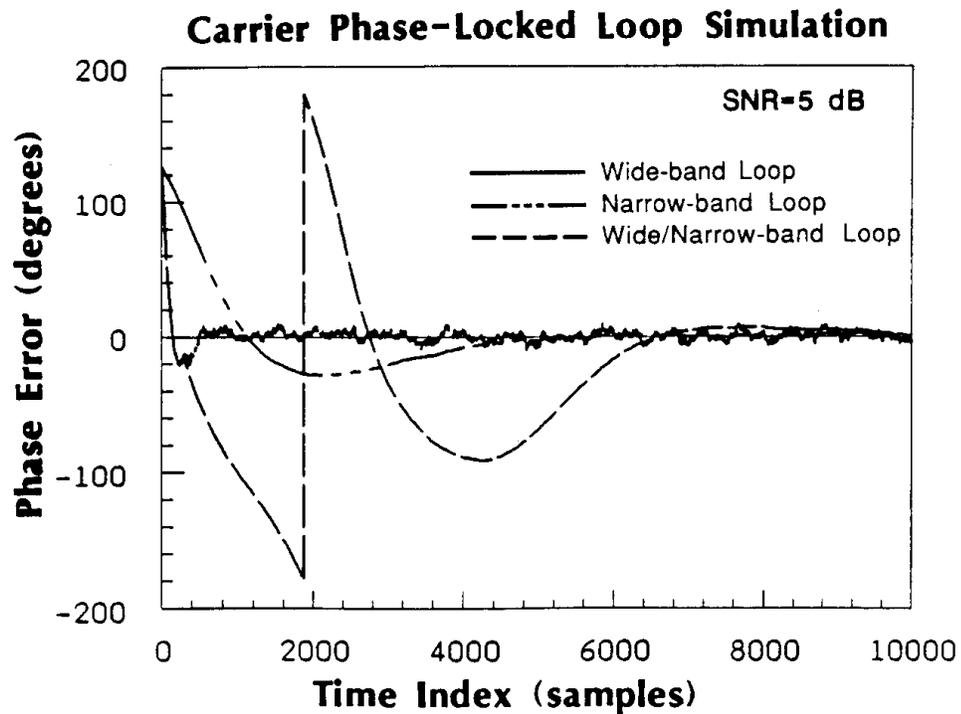
FIGURE 7. CYCLE SLIPPING PHENOMENON IN THE MULTIPLE BANDWIDTH LOOP SIMULATION.
