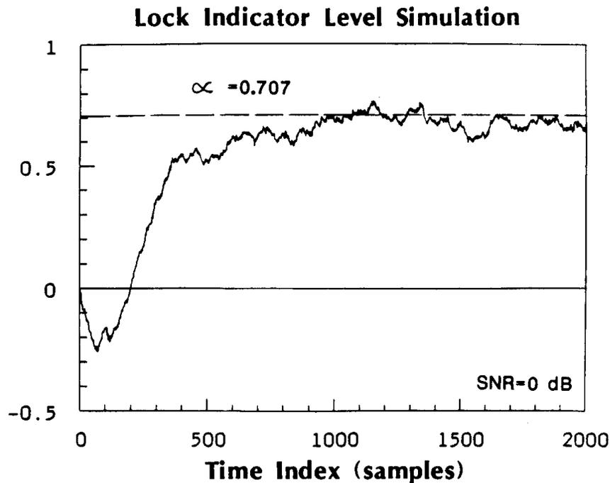
**FIGURE 4. INFLUENCES OF NONCOHERENT AGC ON THE LOCK INDICATOR LEVEL.**
