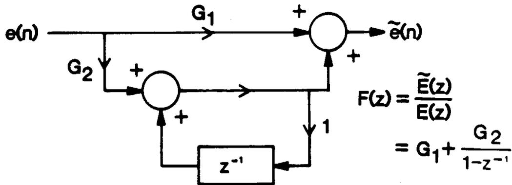
**FIGURE 3. DISCRETE LOOP FILTER FOR A HIGH GAIN LAG-LEAD LOOP.**
