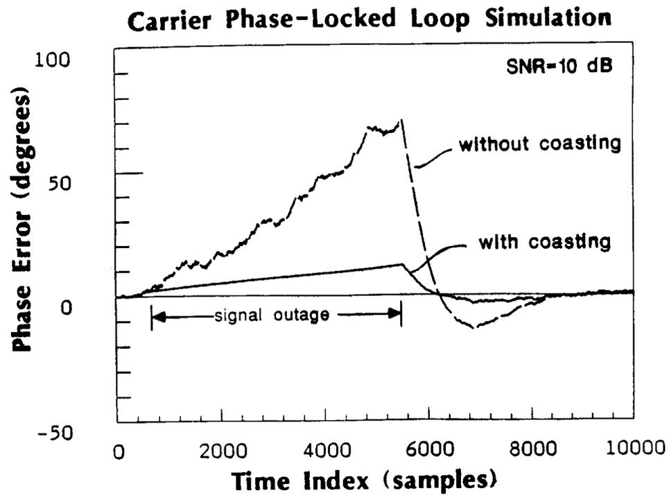
FIGURE 9. COASTING OF THE CARRIER LOOP (PHASE ERROR).
