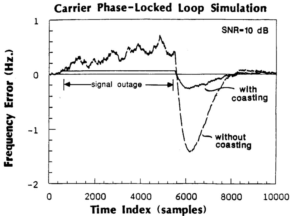
FIGURE 8. COASTING OF THE CARRIER LOOP (FREQUENCY ERROR).
