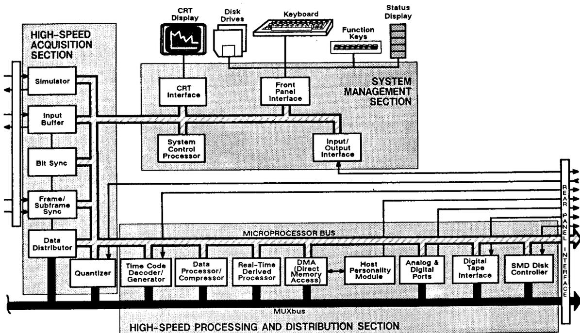
Figure 4. Typical ADS architecture.
