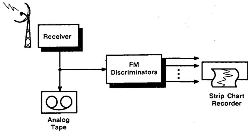
Figure 1. First generation telemetry ground station.
