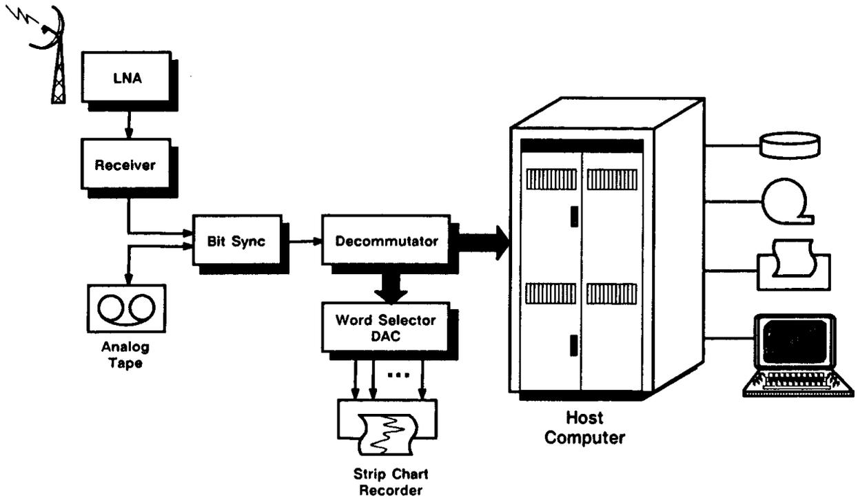
Figure 2. Second and third generation telemetry ground station.
