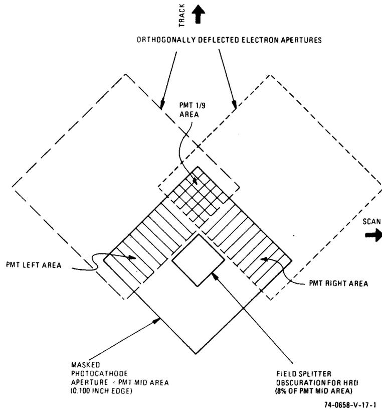
**Figure 2. PMT Detector Aperture**
