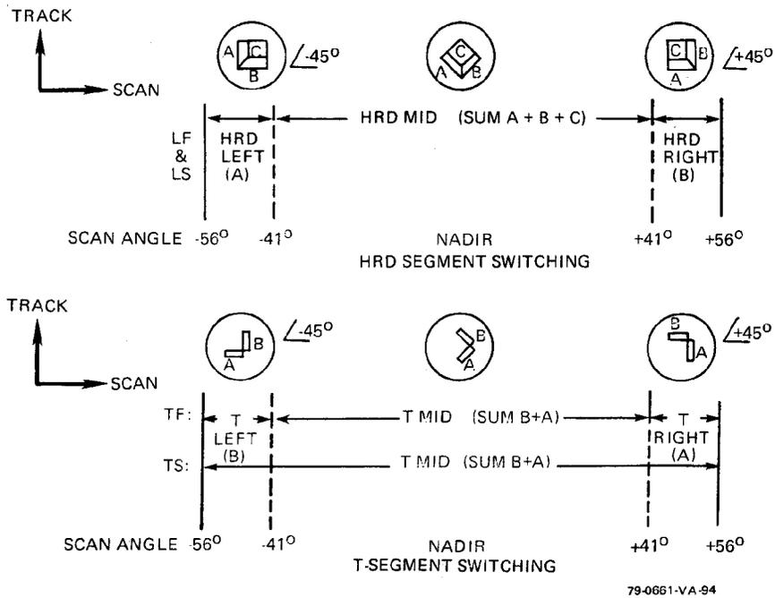
**Figure 3. HRD & T Detector Segment Switching**
