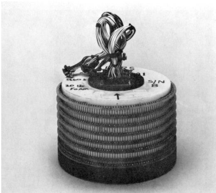
FIGURE 2 STACKED BOARDS PRIOR TO INSTALLATION IN CASE
