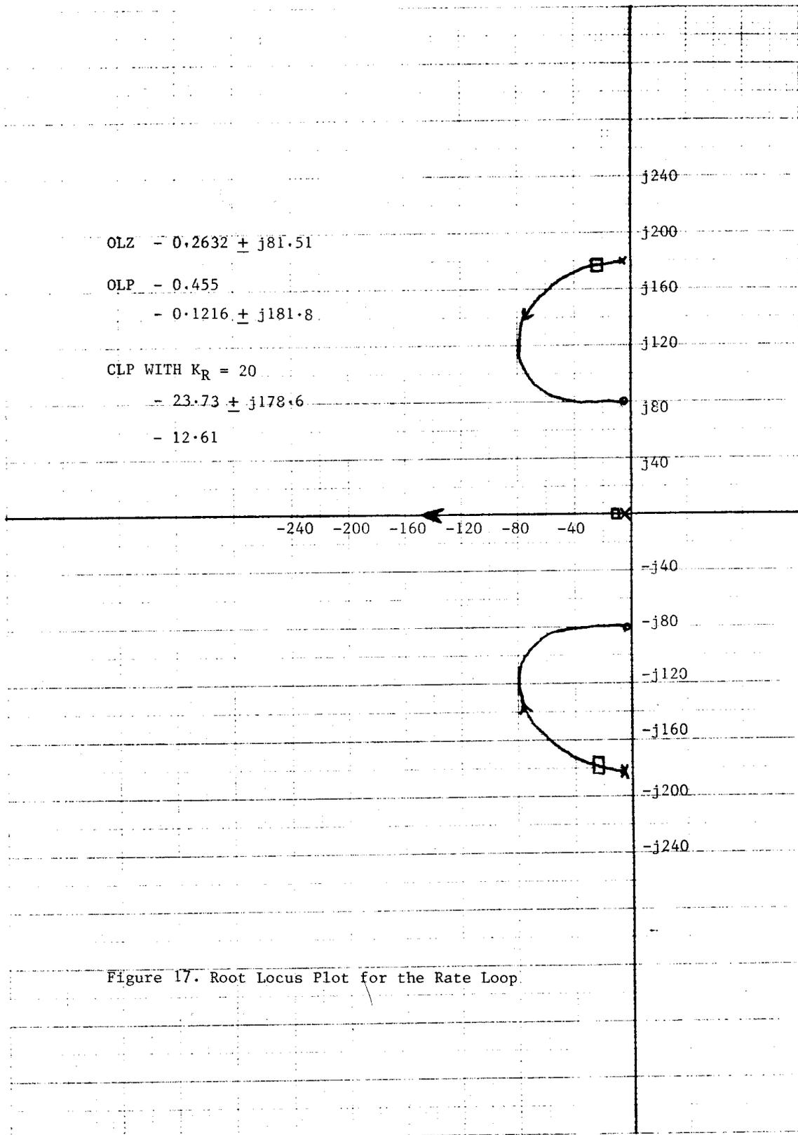
Figure 17. Root Locus Plot for the Rate Loop.
