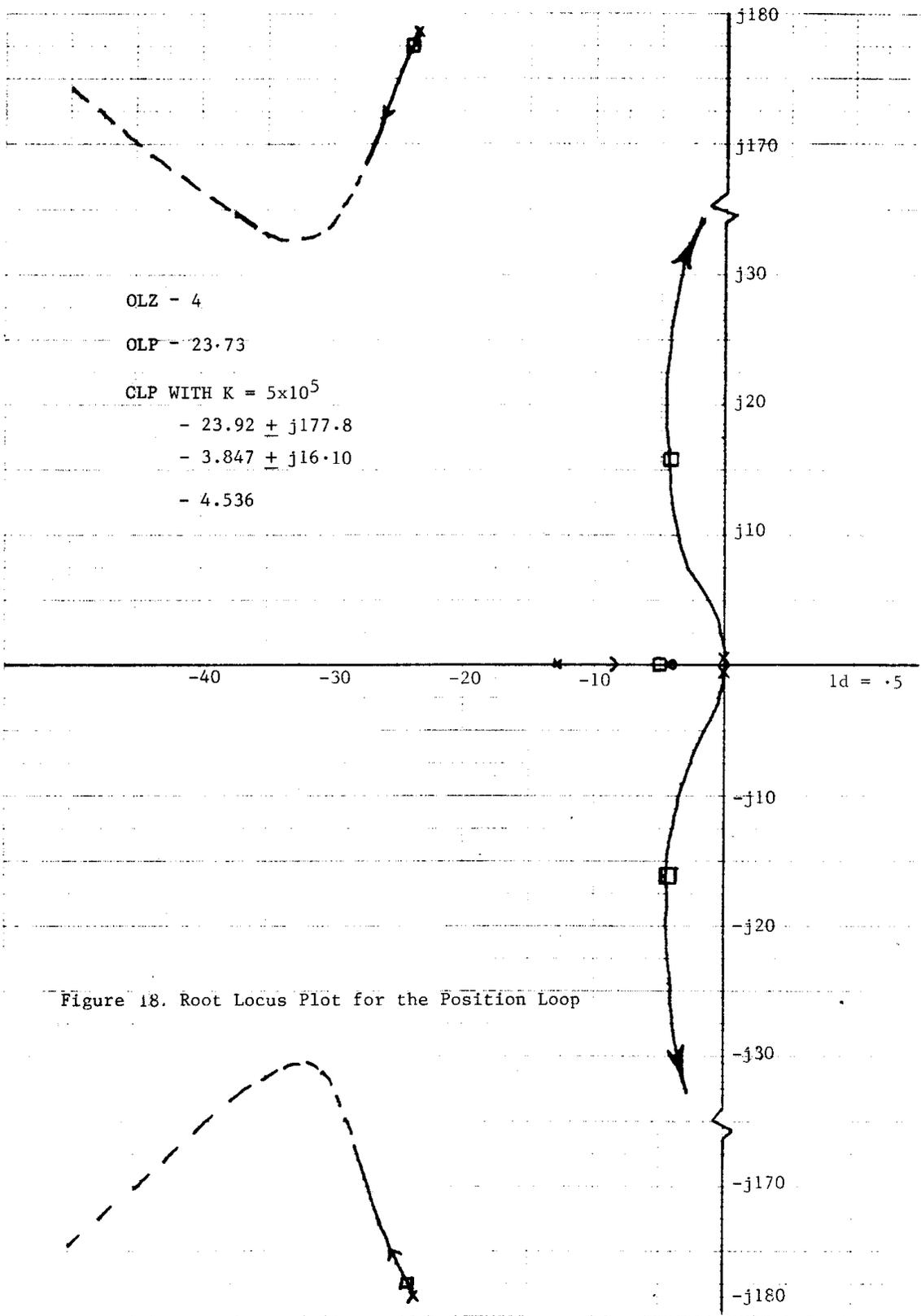
Figure 18. Root Locus Plot for the Position Loop
