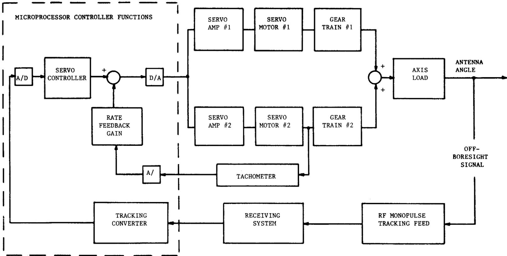
Figure 11. Autotracking Control System-Simplified Block Diagram for One Axis
