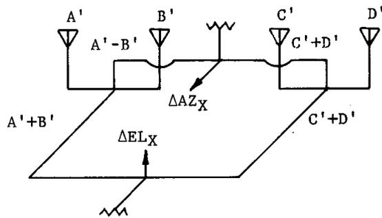
**Figure 6. Dual Band Feed Horns and Waveguide Comparators for Sum (  $\Sigma$  ) and Difference (  $\Delta$  ) Channels**
