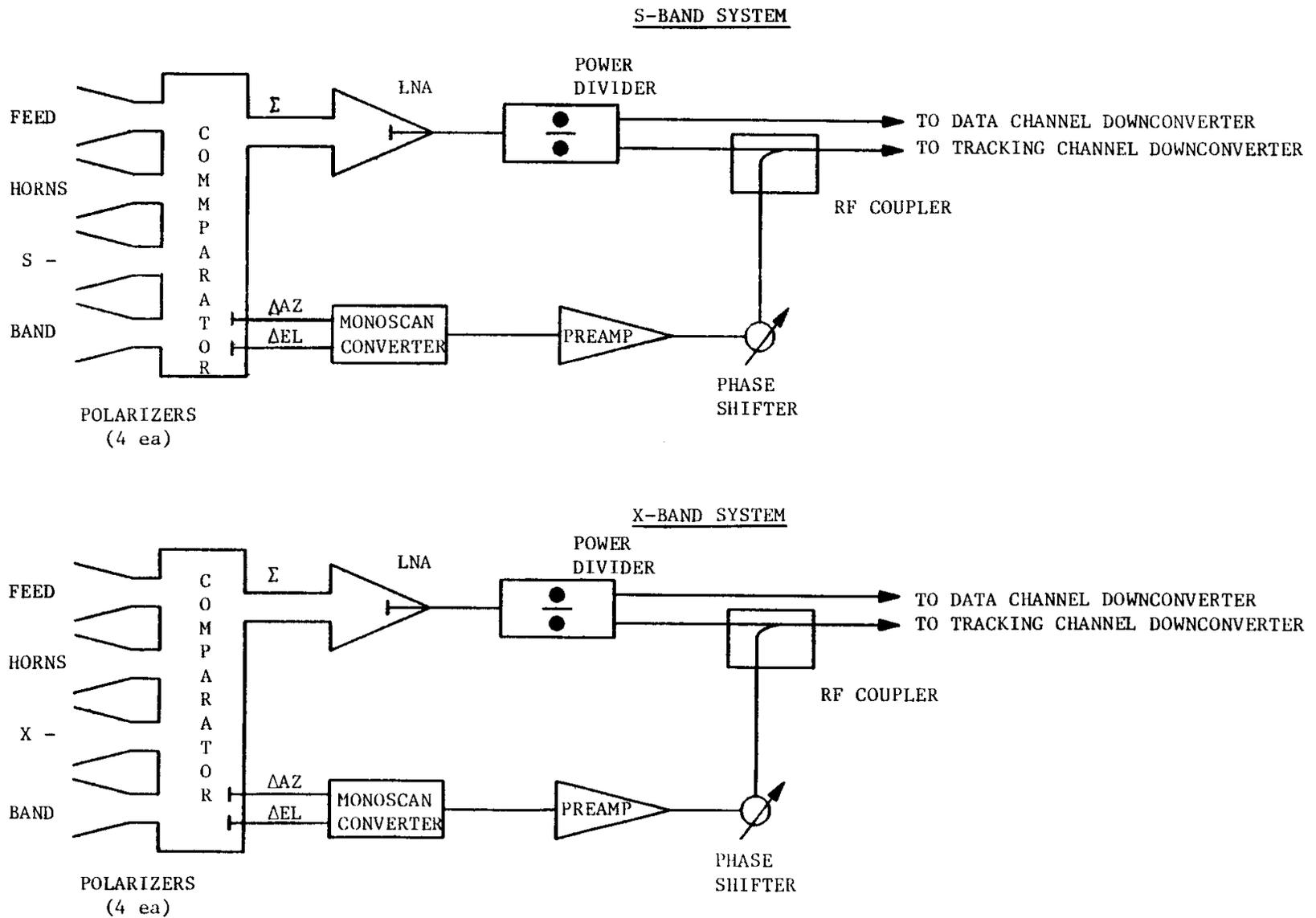
**Figure 4. S-Band & X-Band Telemetry & Tracking Feed Block Diagram**
