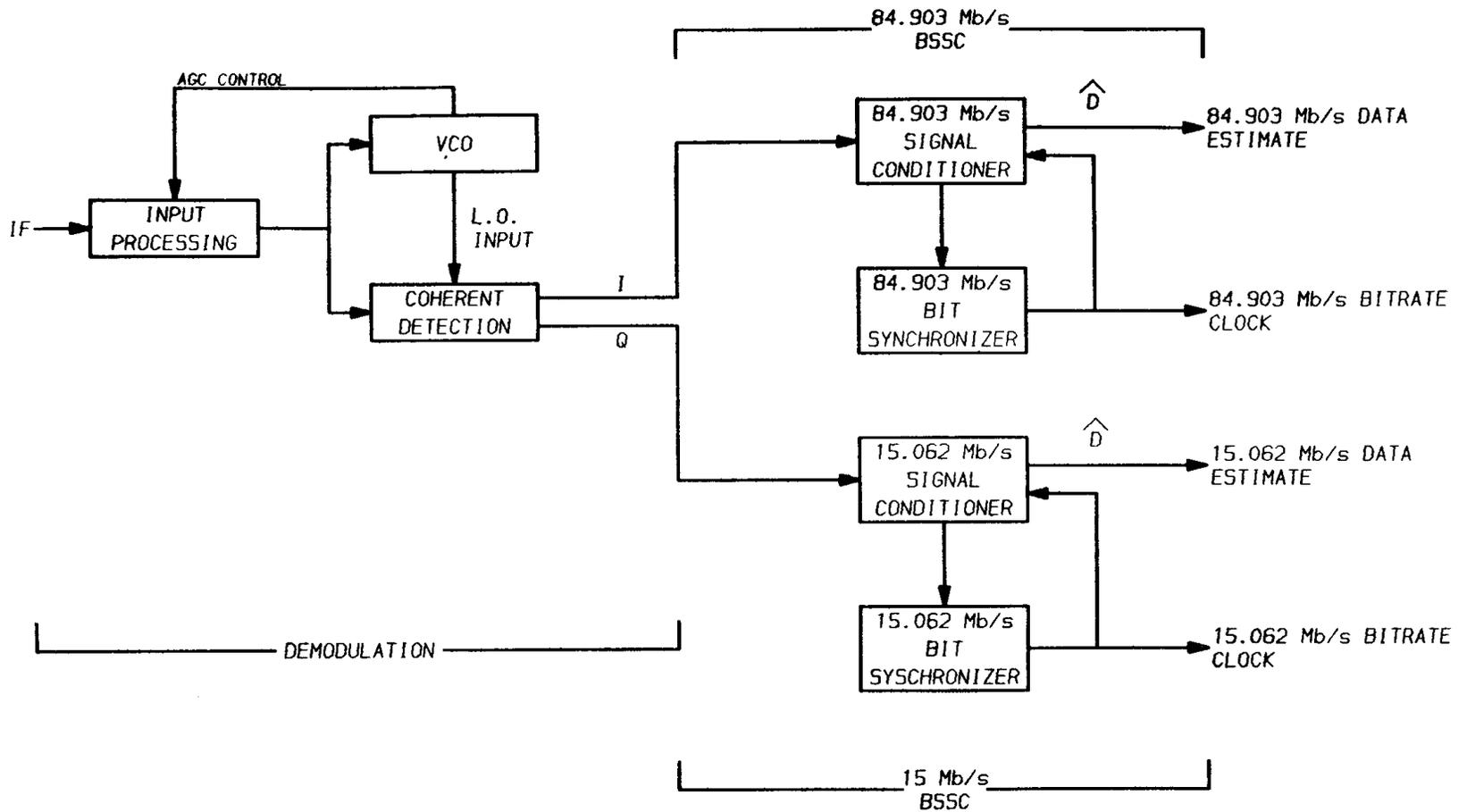
**Figure 10. LANDSAT X-Band Data Receiver/Demodulator**
