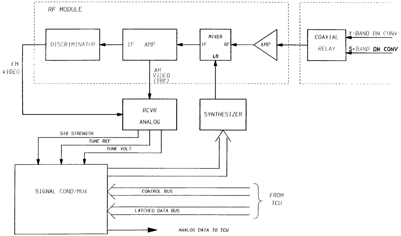
**Figure 9. Tracking Receiver Block Diagram**
