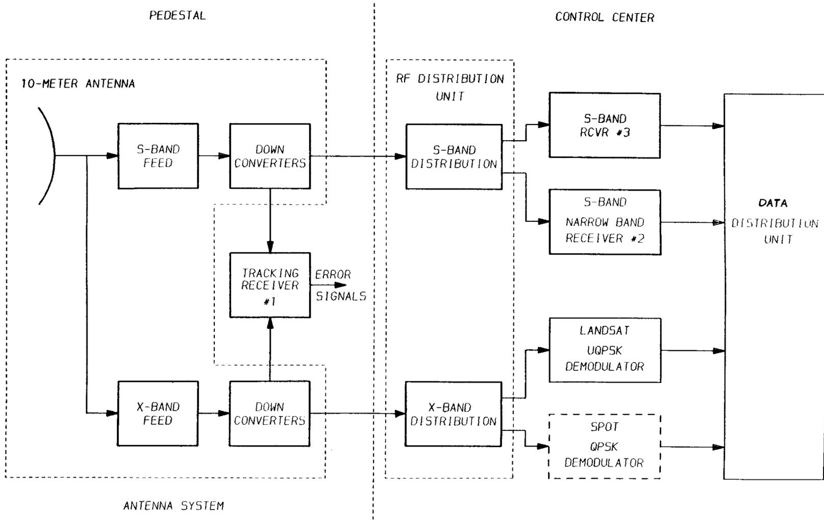
**Figure 8. Receiver System Block Diagram**
