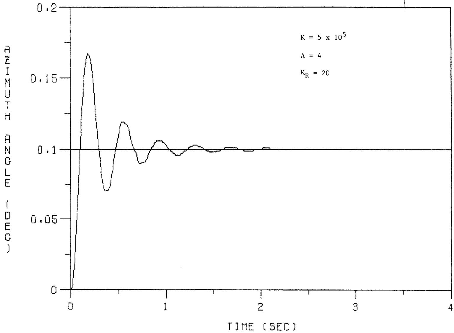
Figure 19. Azimuth Response to Step Input
