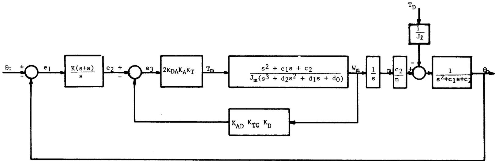
Figure 16. Mathematical Block Diagram of Landsat Control System
