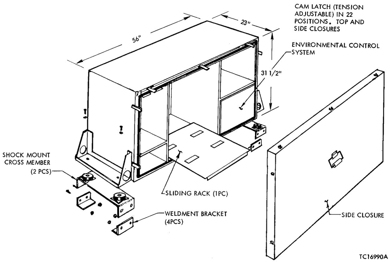
**Figure 10. Airconditioning Equipment Enclosures**
