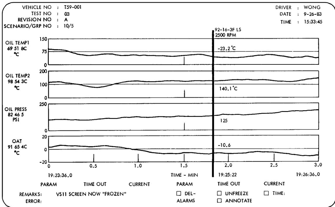
**Figure 14. Stacked Four Curve Scrolling EU Display**
