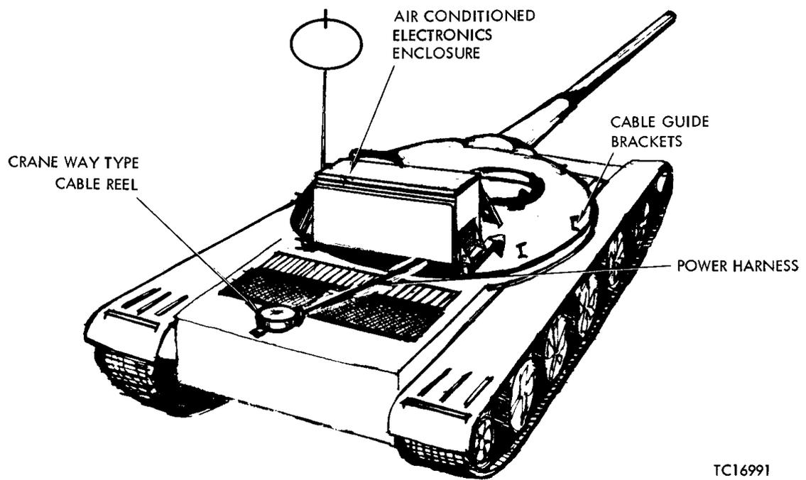
**Figure 5. Externally Mounted Electronics Configuration**
