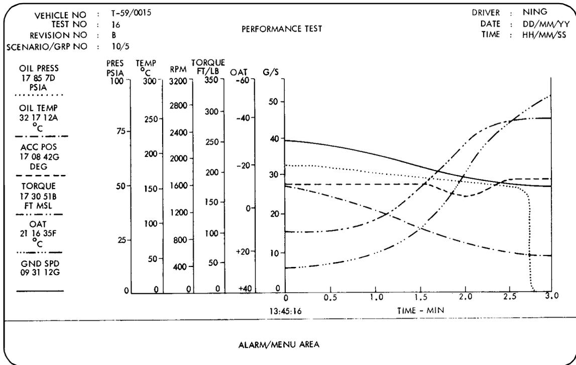
**Figure 15. Overlaid Disk Curve Scrolling EU Display**
