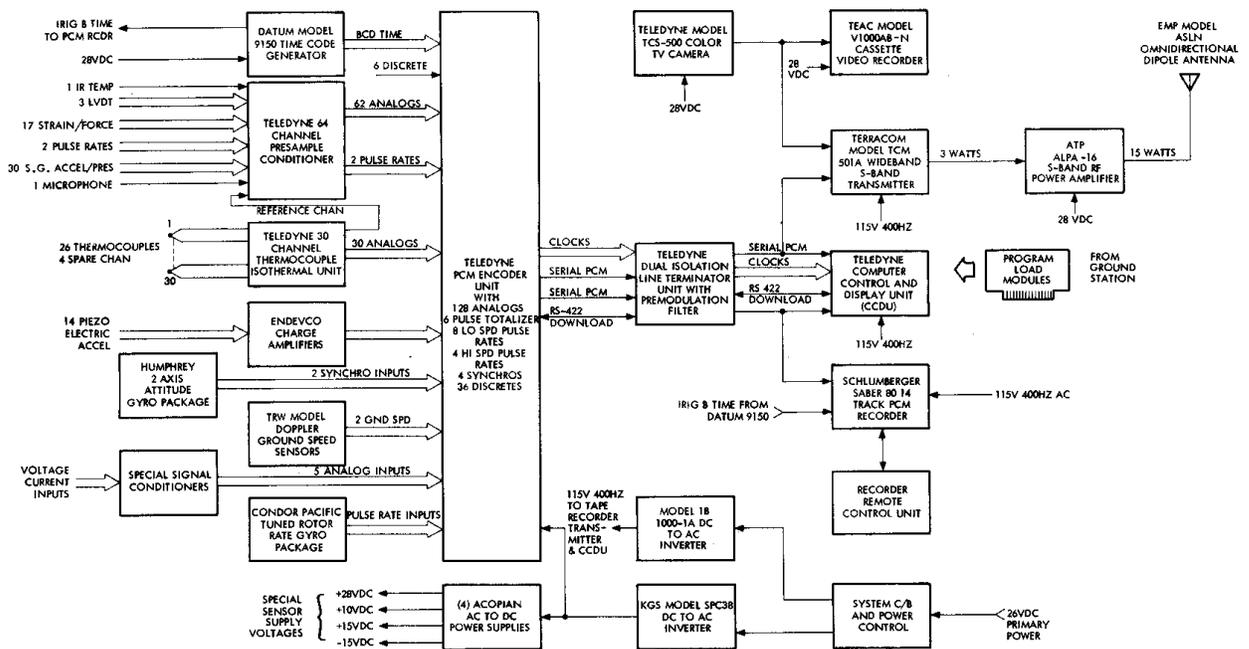
Figure 9. Vehicle-Borne Data Acquisition System Functional Block Diagram
