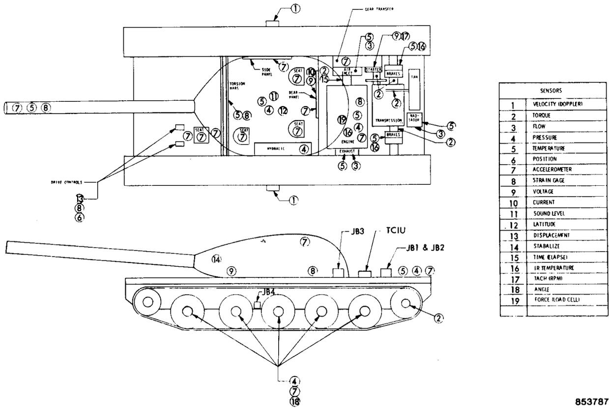
Figure 8. Test Vehicle Sensor Location
