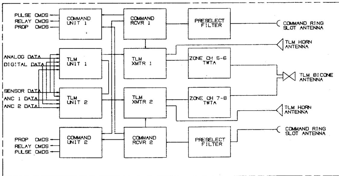
**TELEMETRY, COMMAND AND RANGING SUBSYSTEM
