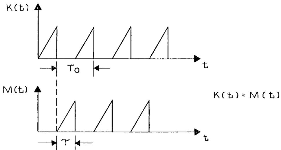
**FIGURE 1** DISPLACEMENT AT WHICH THE CORRELATION IS ZERO
