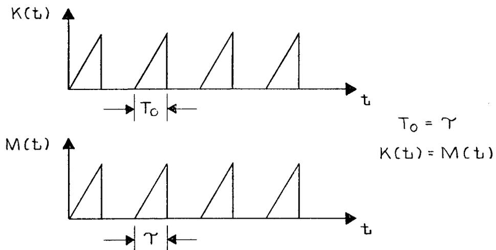
**FIGURE 2** DISPLACEMENT AT WHICH THE CORRELATION IS A MAXIMUM
