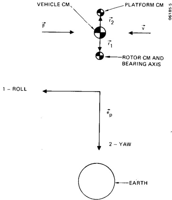
Figure 7. Mass Center and Spin Axis Positions in Steady State Pointing
