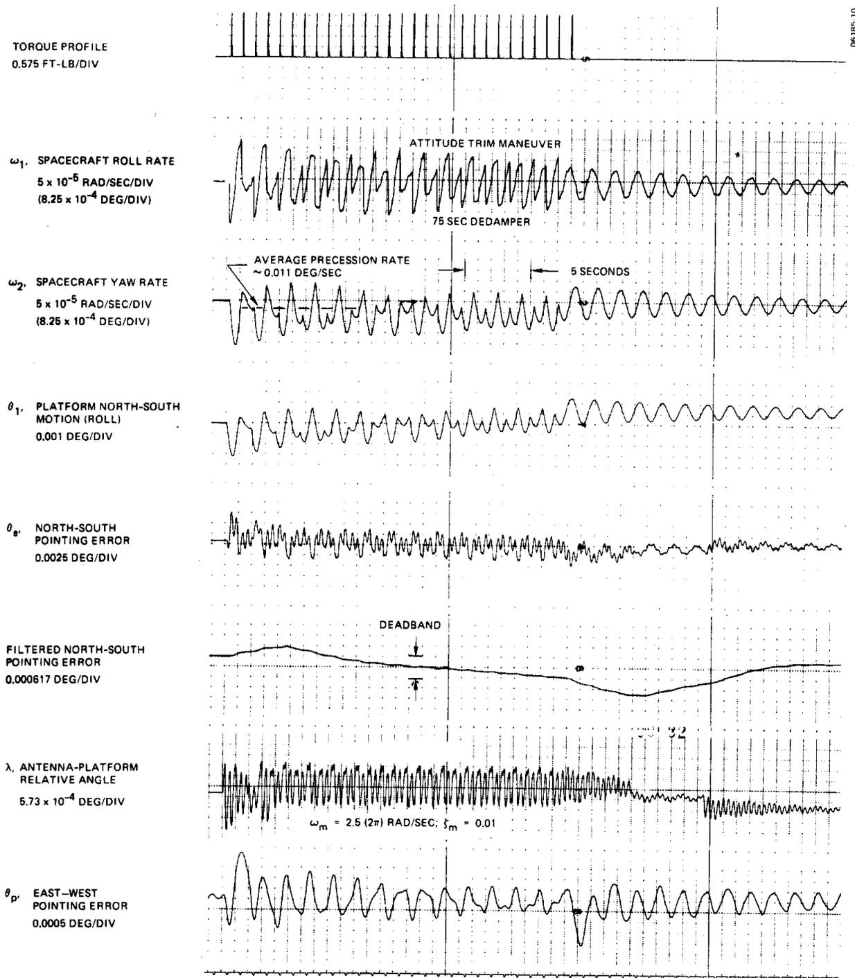
**Figure 5. Vehicle Dynamics During Attitude Trim Maneuver**
