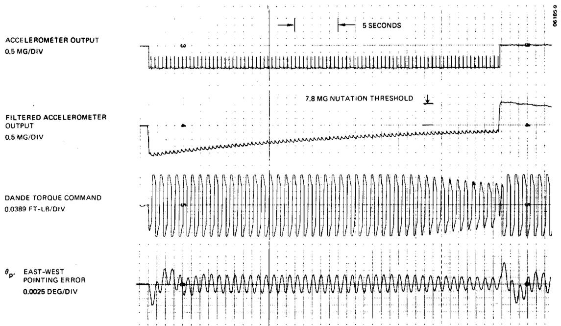
**Figure 9b. Vehicle Dynamics During North-South Velocity Maneuver**
