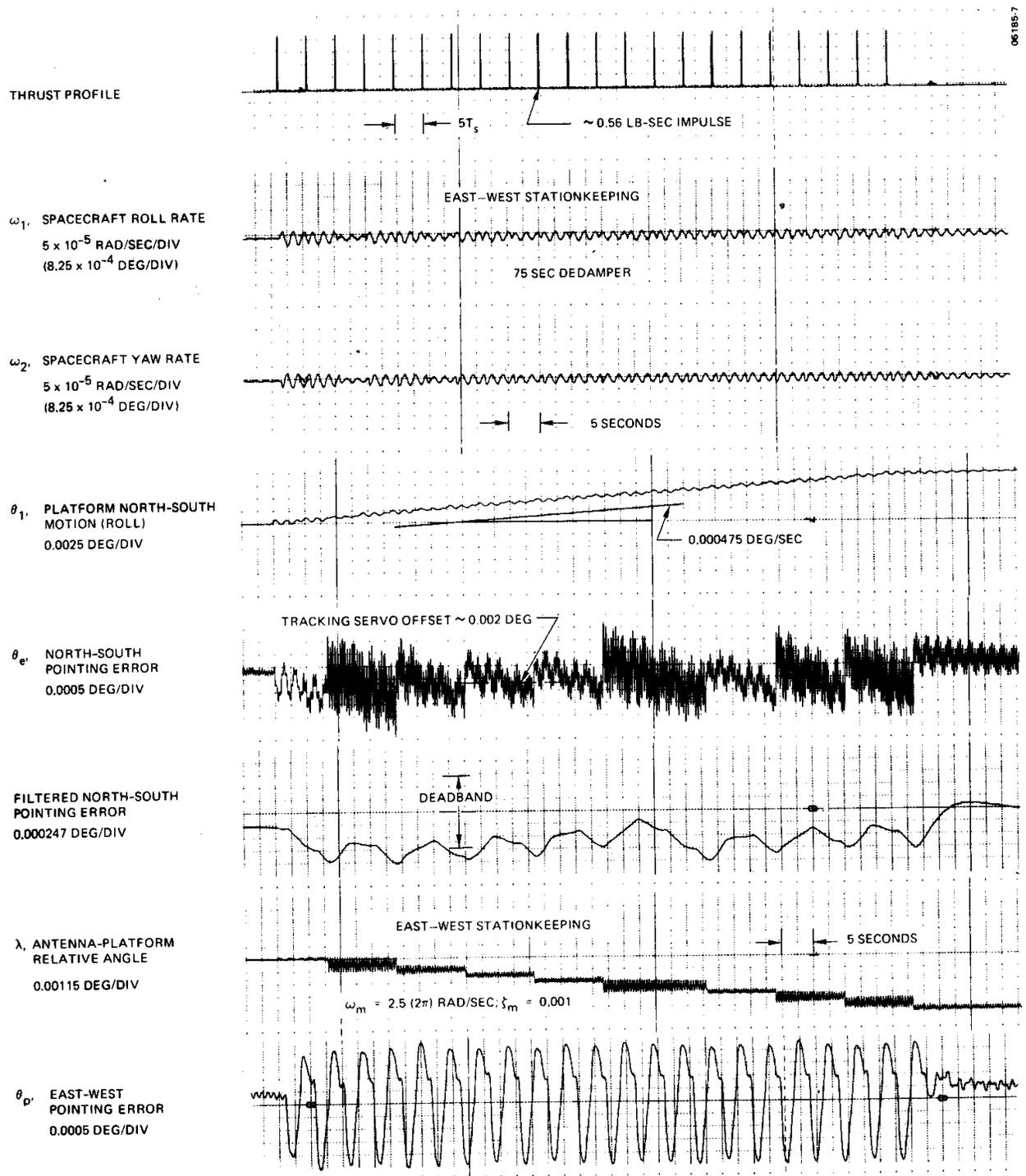
Figure 6. Vehicle Dynamics During East-West Velocity Maneuver
