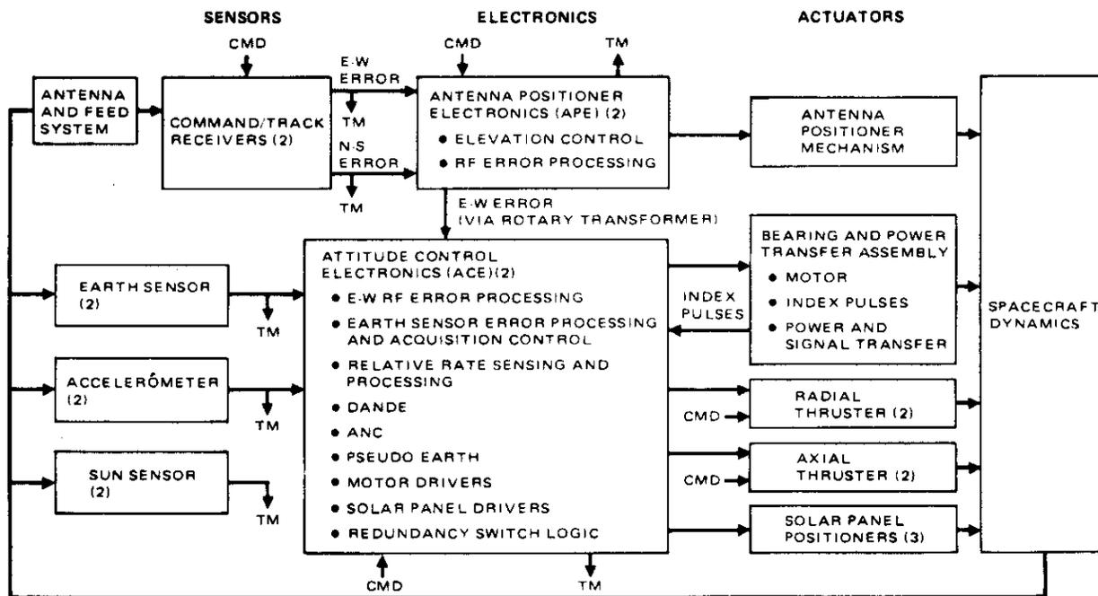
Figure 2. Attitude Control System Functional Block Diagram
