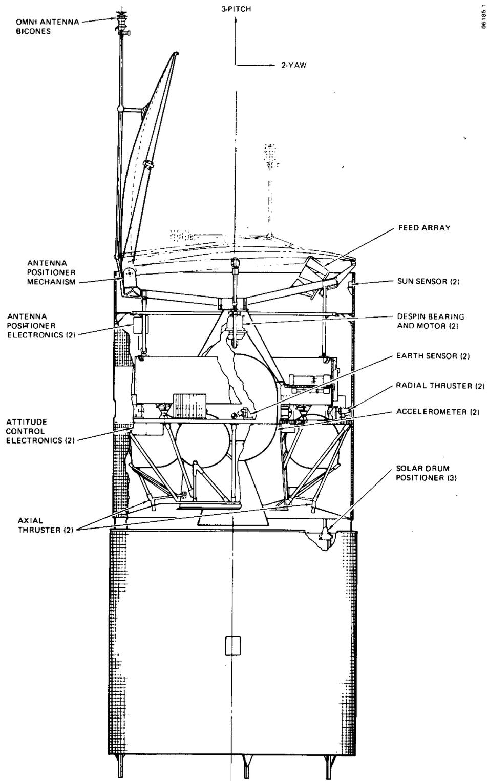
**Figure 1. Spacecraft Configuration and Control Element Location**
