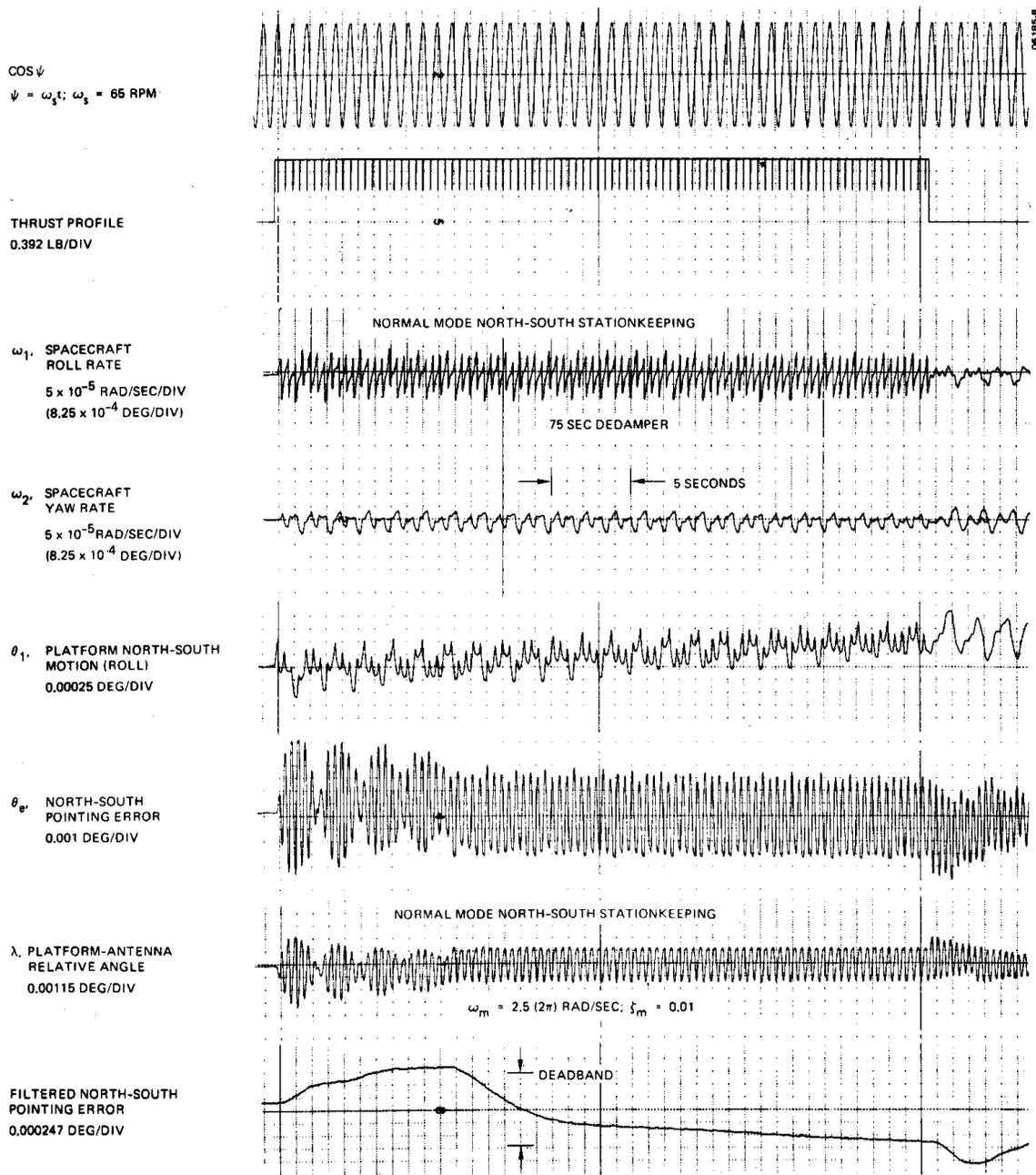
**Figure 9a. Vehicle Dynamics During North-South Velocity Maneuver**
