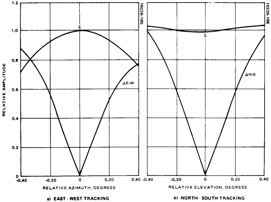
**Figure 4. Beacon Error Sensor Characteristic**
