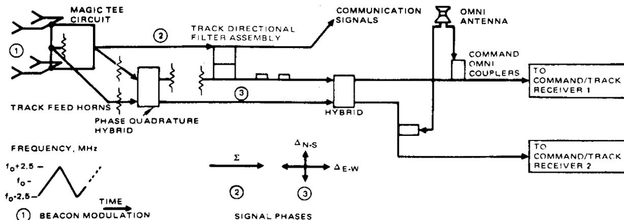
Figure 3. RF Beacon Track Network Schematic
