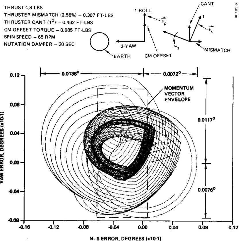
Figure 8. Motion of Spin Axis on an Inertial Plane During North-South Velocity Maneuver
