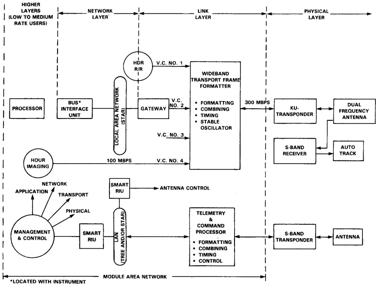
**Figure 1. Functional Diagram, Platform Data Flow**
