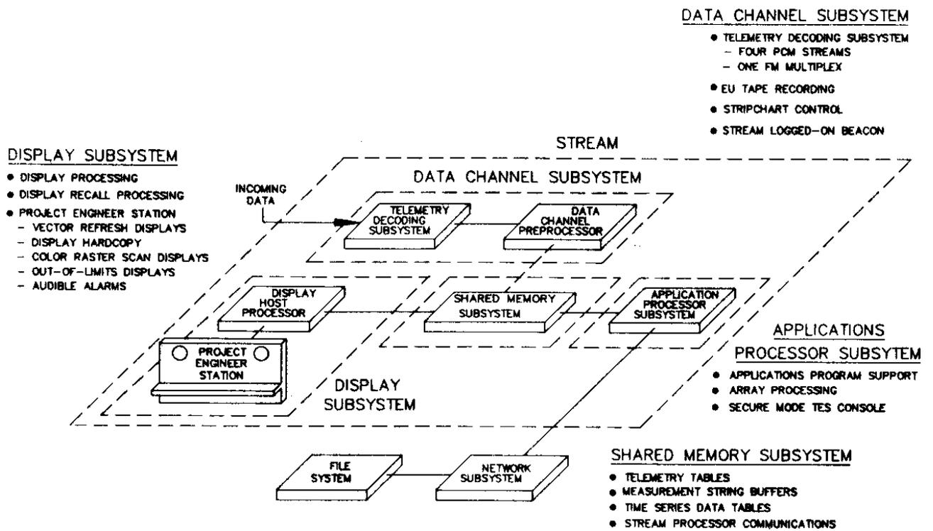
Figure 1. RTPS III System Architecture
