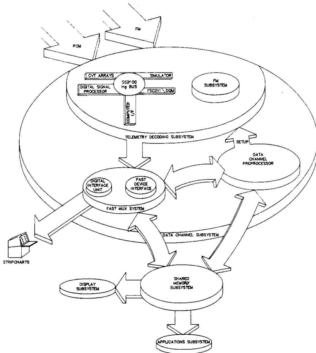
**Figure 2. Data Channel Subsystem
