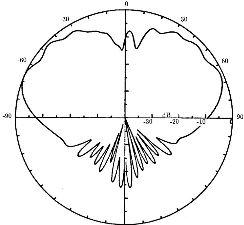
Fig. 5.  $E_0$  radiation pattern for the loaded DC mode in the H-plane of the (0,1) mode.
