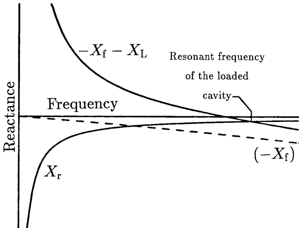
Fig. 1. Reactance components *versus* frequency for determining the resonant frequency of a loaded microstrip antenna.
