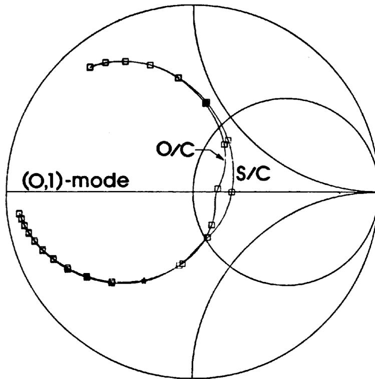
Fig. 3. Input impedance at the (0,1) port with the loaded DC port open and short circuited.
