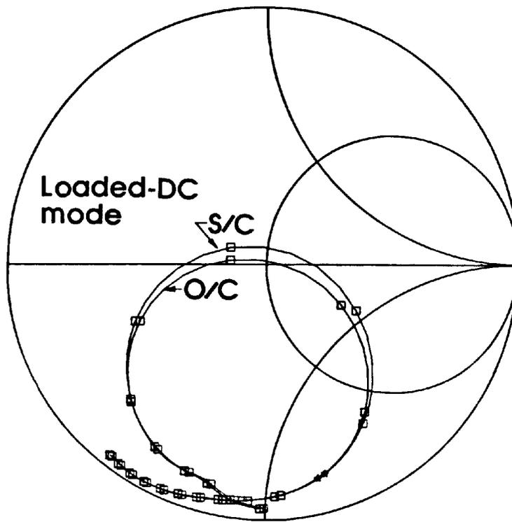
Fig. 4. Input impedance of the loaded DC port with the (0,1) mode port open and short circuited.
