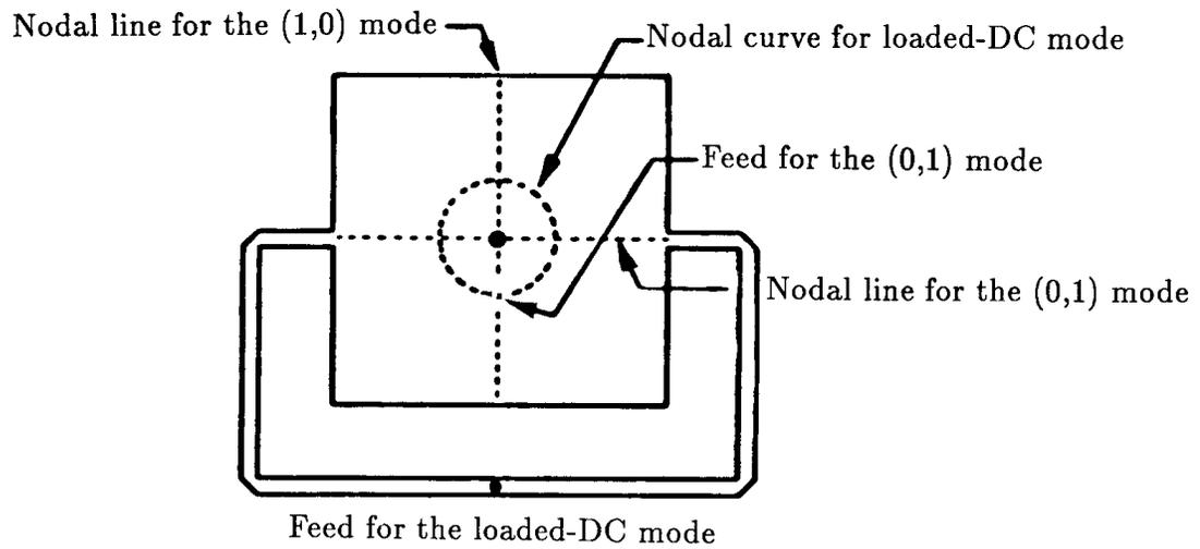
Fig. 2. Geometry of reactively loaded dual mode microstrip antenna.
