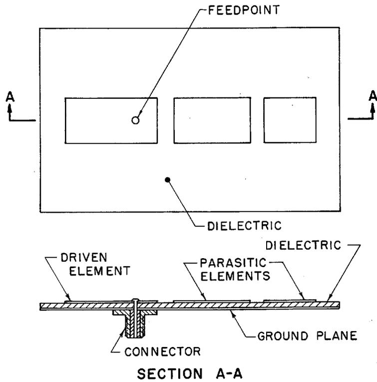
**FIG. 6 THREE ELEMENT PARASITIC ARRAY**
