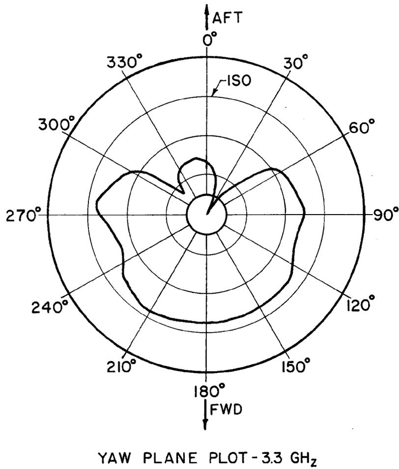
**FIG. 4 TWO ELEMENT PARASITIC ARRAY RADIATION PATTERN**
