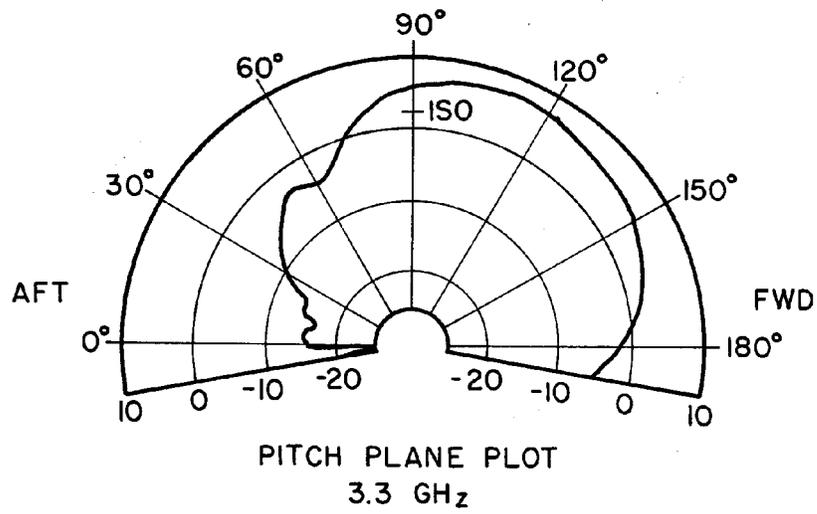
**FIG. 3 TWO ELEMENT PARASITIC ARRAY RADIATION PATTERN**
