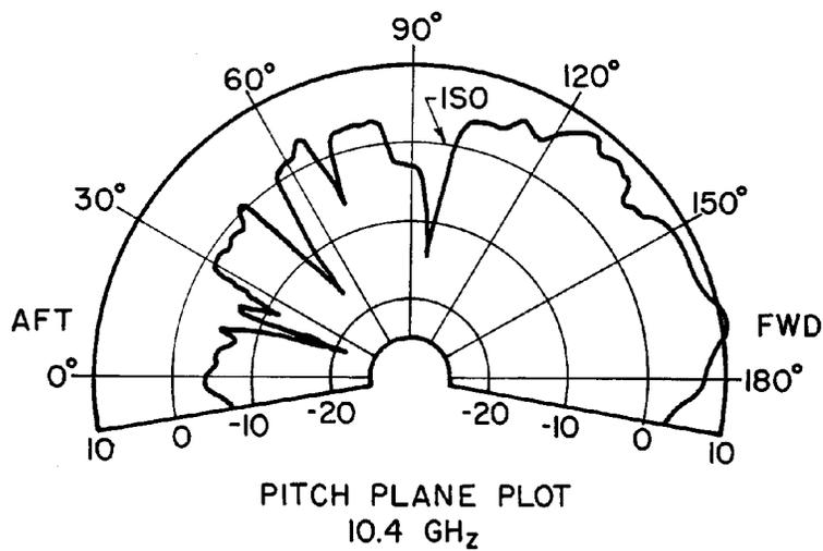
**FIG. 8 THREE ELEMENT PARASITIC ARRAY RADIATION PATTERN**
