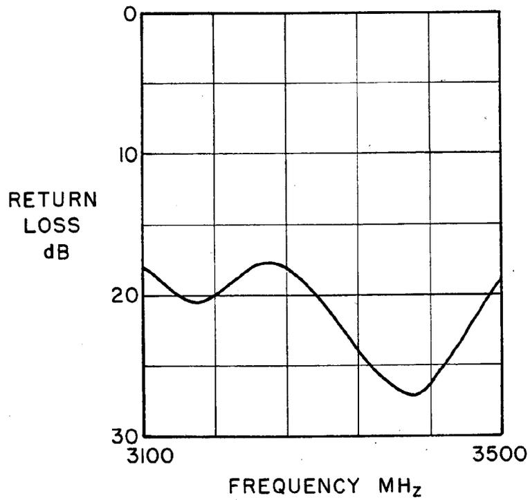
**FIG. 5 TWO ELEMENT PARASITIC ARRAY RETURN LOSS VS FREQUENCY**
