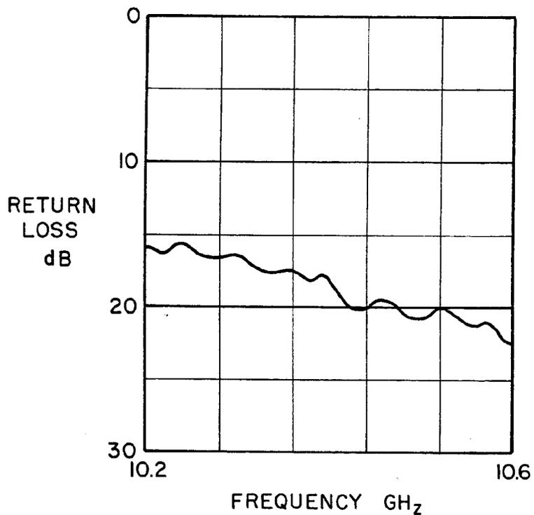
**FIG. 7 THREE ELEMENT PARASITIC ARRAY RETURN LOSS VS FREQUENCY**
