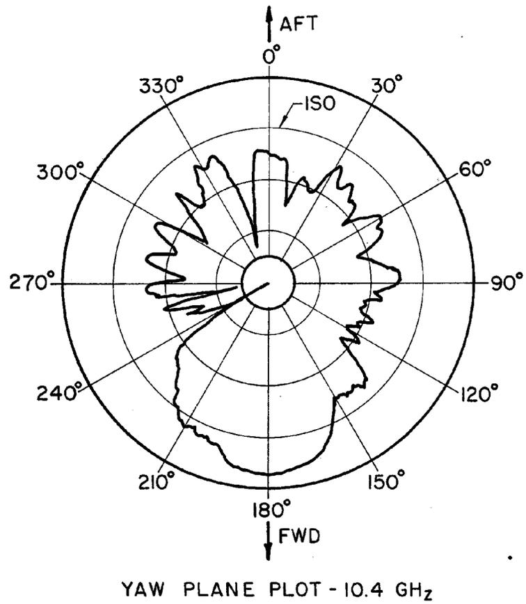
**FIG. 9 THREE ELEMENT PARASITIC ARRAY RADIATION PATTERN**
