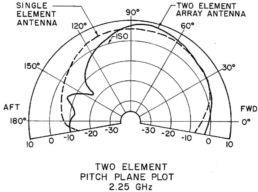
**FIG. 2 RADIATION PATTERN COMPARISON BETWEEN A SINGLE ELEMENT AND A TWO ELEMENT ARRAY**
