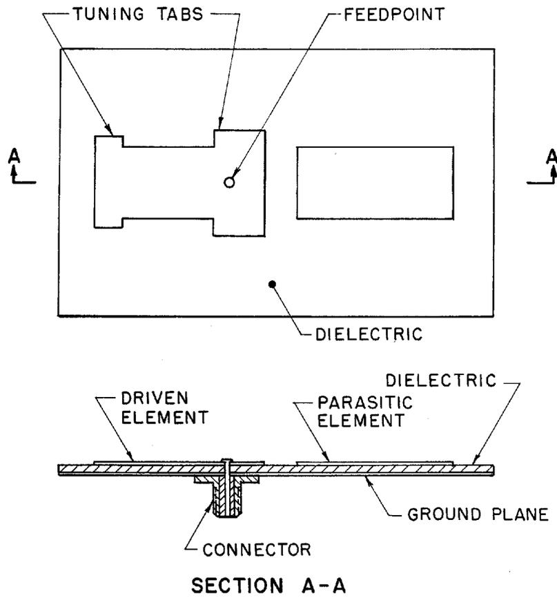
**FIG. 1 TWO ELEMENT PARASITIC ARRAY**
